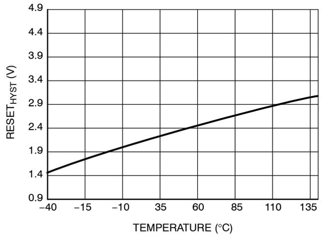
Figure 16. V<sub>CC(LATCH)</sub>-V<sub>CC\_HYST</sub> vs Temperature
