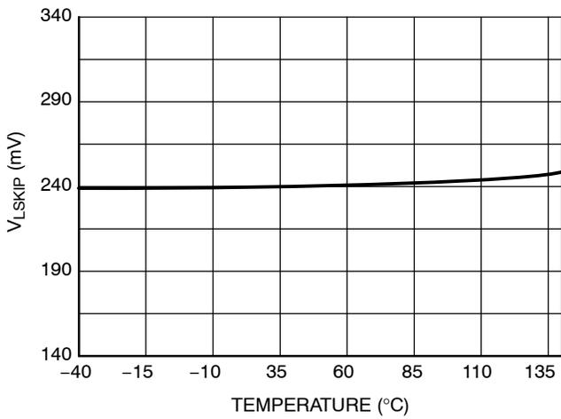
Figure 23. Skip Level vs. Temperature
