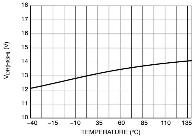
Figure 22. Drive Voltage V<sub>DRV(HIGH)</sub> vs Temperature
