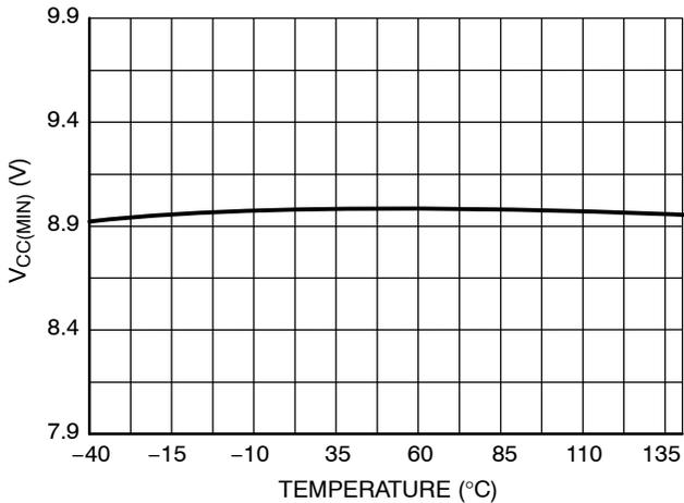
Figure 13. V<sub>CC(MIN)</sub> Voltage vs Temperature
