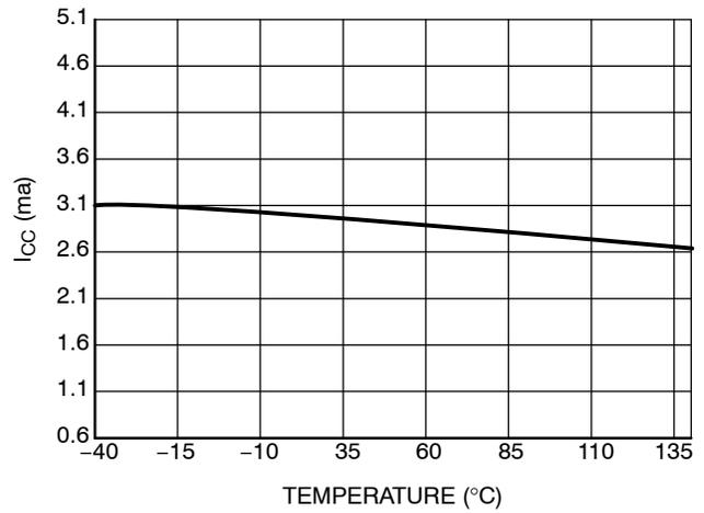
Figure 4. I<sub>CC2</sub> vs. Temperature
