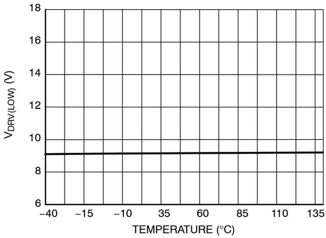
Figure 21. V<sub>DRV(LOW)</sub> vs Temperature
