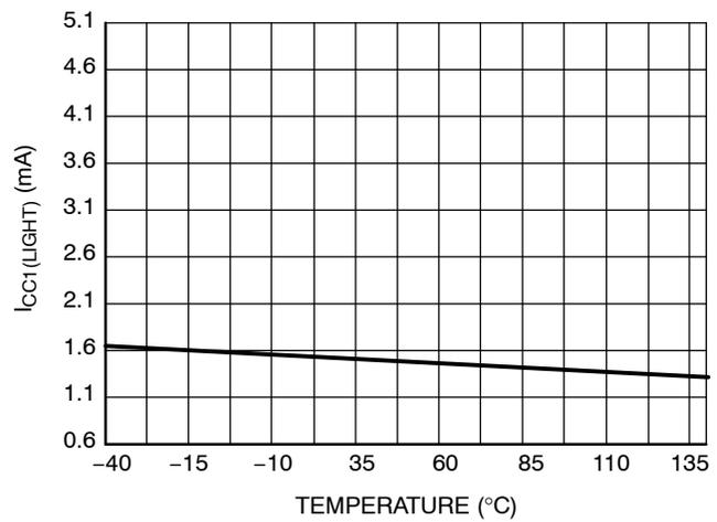
Figure 18. I<sub>CC1(LIGHT)</sub> vs Temperature
