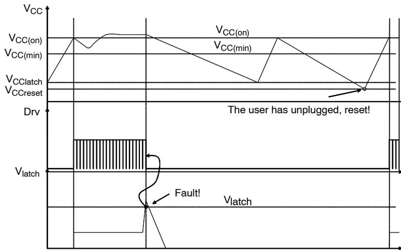
**Figure 40. The Part is Reset when V<sub>CC</sub> Reaches 5 V or when BO Senses the Bulk Capacitor Voltage is Back to Normal**
