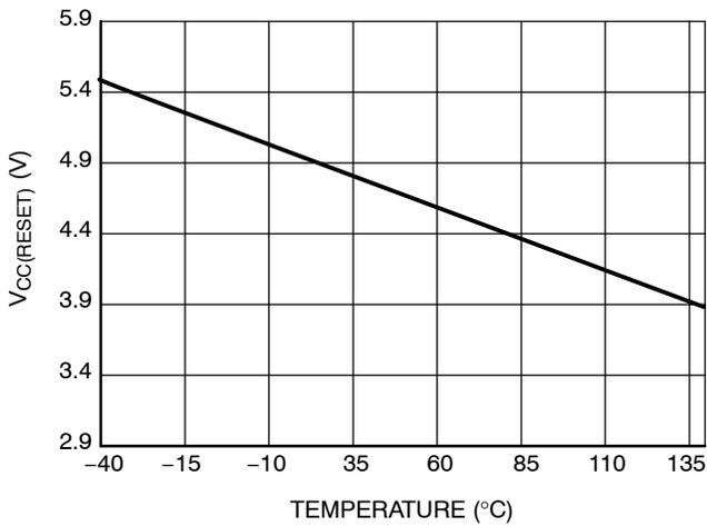
Figure 15. V<sub>CC(RESET)</sub> vs Temperature
