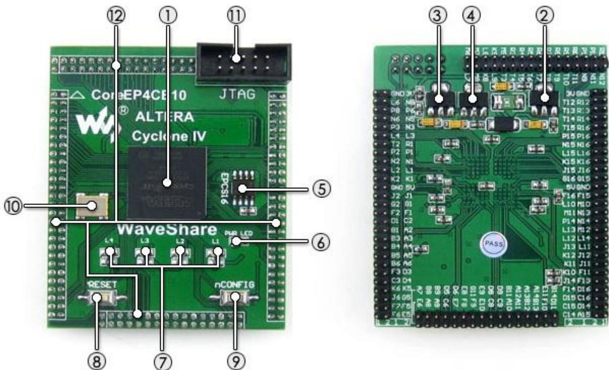
1. EP4CE10F17C8N: the ALTERA Cyclone IV FPGA device which features:
