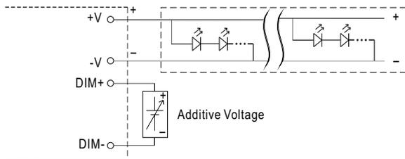
"DO NOT connect "DIM- to -V"
