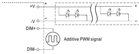
"DO NOT connect "DIM- to -V"
