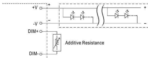
"DO NOT connect "DIM- to -V"
