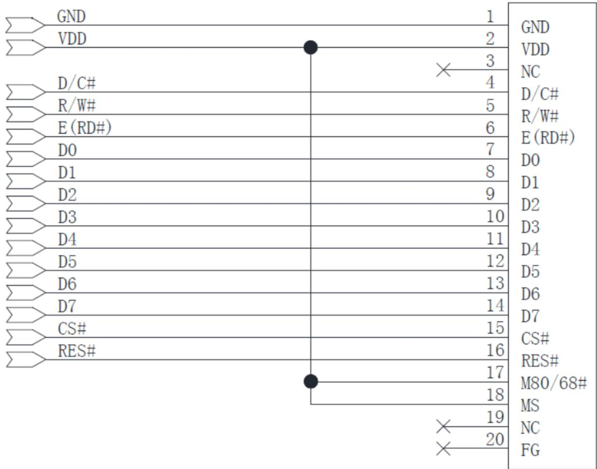
Pin connected to MCU interface: D[0:7], E(RD#), R/W#, RES#, D/C#, CS#.
