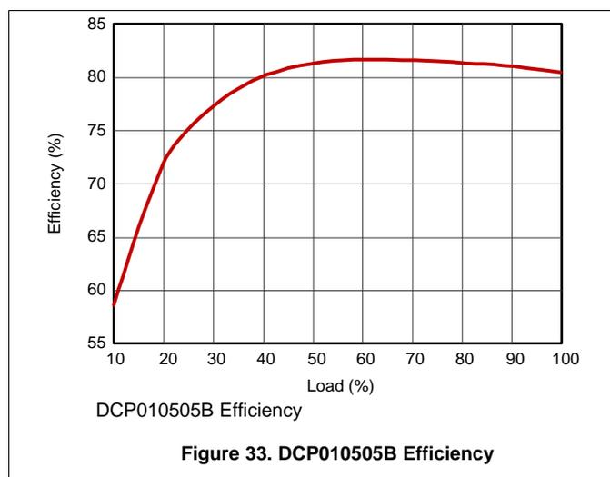
Figure 33. DCP010505B Efficiency
