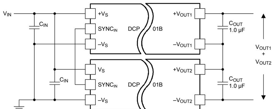
Figure 29. Multiple DCP01B Devices Connected in Series
