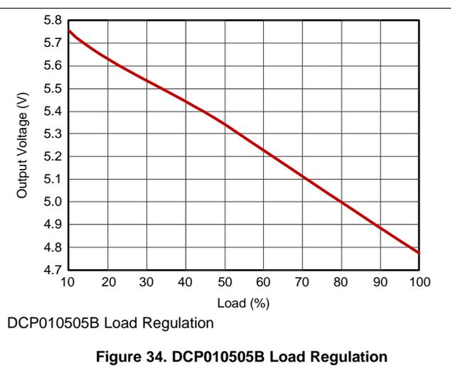
Figure 34. DCP010505B Load Regulation
