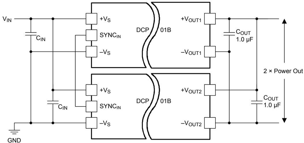
Figure 31. Multiple DCP01B Devices Connected in Parallel
