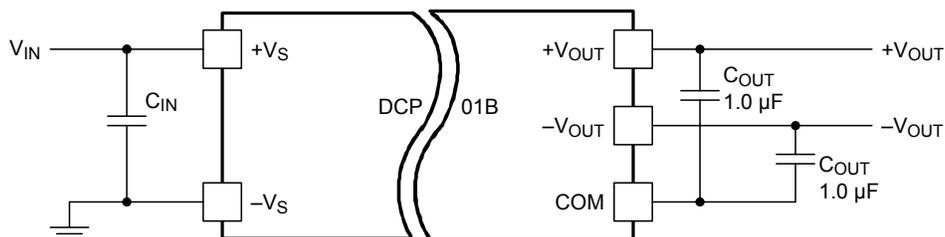
Figure 30. Dual Output Devices Connected in Series
