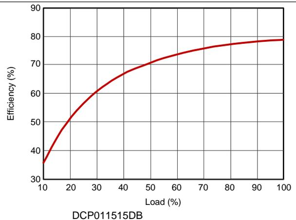
Figure 24. Efficiency vs Load
