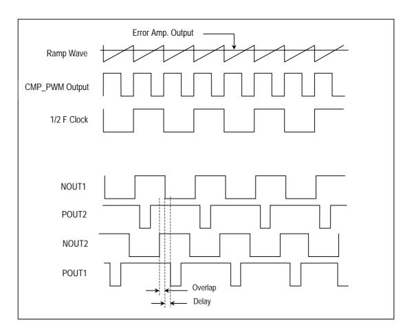
If the lamp operation frequency is set to higher than resonant frequency of the LC tank, symmetry ZVS switching operation can be performed. A well-controlled delay and overlap timing relationship play the key role of this control scheme. It can be set through using proper resistor connected on RTDLY pin. (Patent pending)
