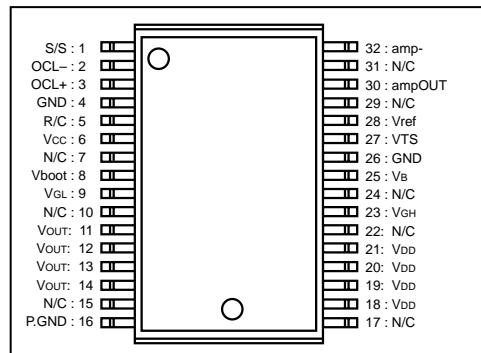
■ **Vref** - Temperature compensated internal voltage. You can pull 1mA maximum for external circuit.
