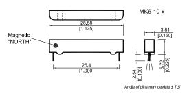
\* MK6-10-E is a magnetic latching sensor which is opened or closed by a passing magnet and remains in that state until a magnet of opposite polarity or direction passes by again. The E refers to a latching sensor and does not represent the magnetic sensitivity.
