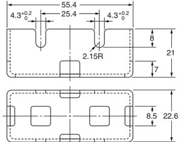
Note: The Cover has six holes for easy lead wire connections.
