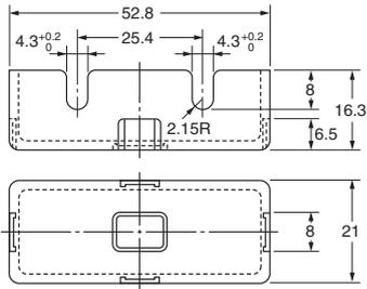
Note: The Cover has five thin, easy-to-separate portions for easy lead wire connections.
