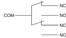
Note: The NO and NC terminal arrangement is reversed for Models with reverse operation (Z-10FM).
