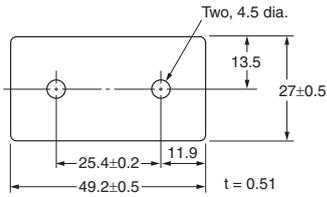
Note: 1. Each dimension has a tolerance of  $\pm 0.4$  mm unless otherwise specified.
