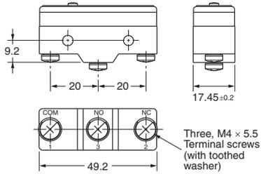
Note: With reverse action models (Z-15GM), the positions of NO and NC terminals are reversed.
