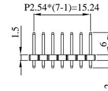
The non-specified tolerance of dimension is ±0.3 mm .
