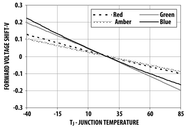
Figure 13. Forward Voltage Shift vs Junction Temperature
