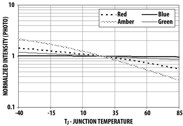
Figure 12. Relative Intensity Shift vs Junction Temperature
