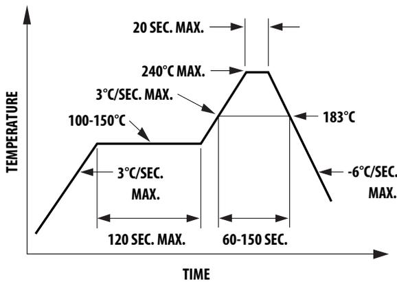
Figure 16. Recommended Lead Reflow Soldering Profile
