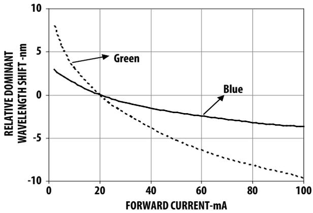
Figure 10. Dominant Wavelength Shift vs Forward Current
