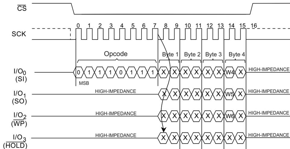
The Set Burst with Wrap instruction sequence is:  $\overline{CS}$  goes low → Send Set Burst with Wrap instruction → Send 24 Dummy bits → Send 8 “Wrap bits” →  $\overline{CS}$  goes high.
