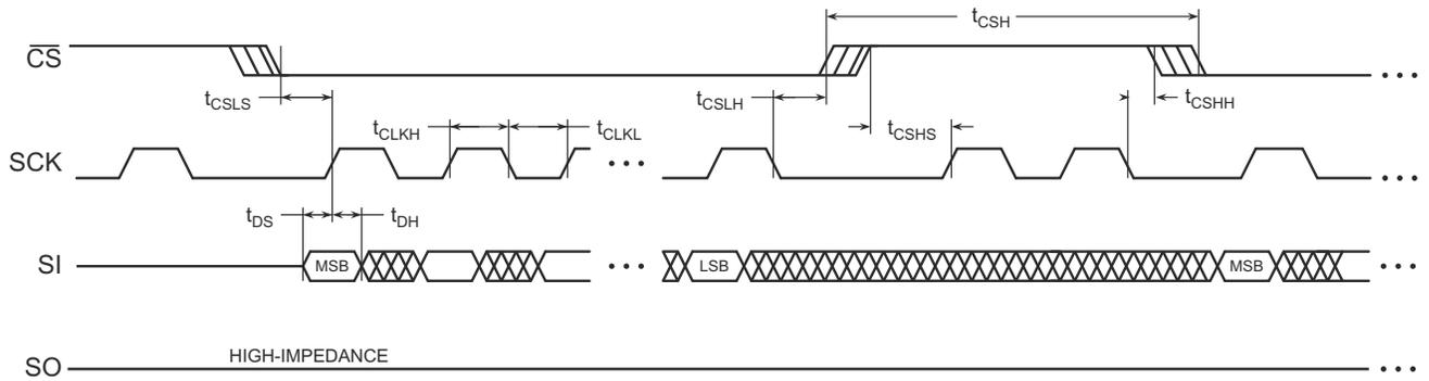
Figure 14-2. Serial Output Timing
