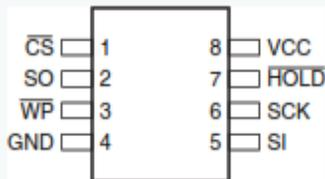
Figure 2-3. 8-UDFN — Top View
