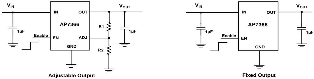
$$V_{OUT} = V_{REF} \left( 1 + \frac{R_1}{R_2} \right) \text{ where } R_2 \leq 80k\Omega$$
