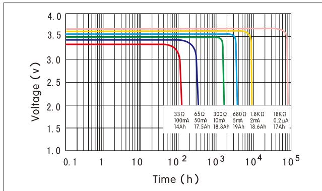
Capacity vs. Current (2.0V cut-off)
