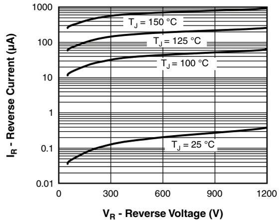
Fig. 2 - Values of Reverse Current vs. Reverse Voltage
