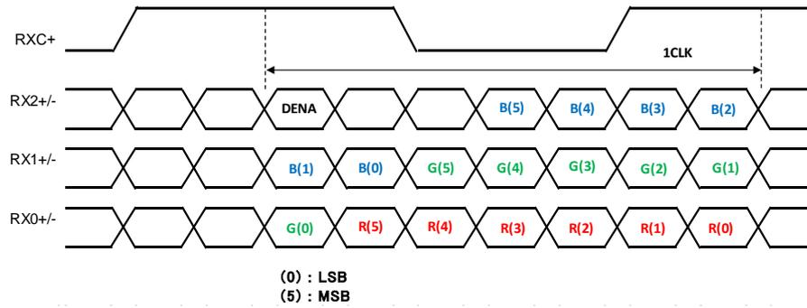
When LVMD is "L" and 6 bit input, the following connection is recommended.
