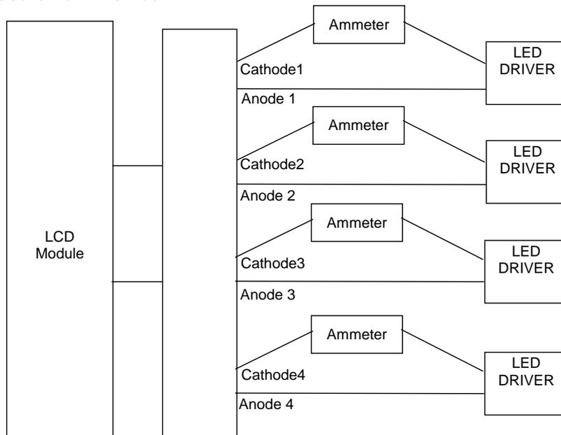
\*3) LED life time is defined as the time when the LCD module brightness becomes 50% compared to the initial value under the measurement condition shown in page 18 and 19.
