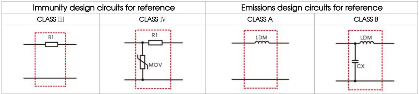
Electromagnetic Compatibility Solution--Recommended Circuit
