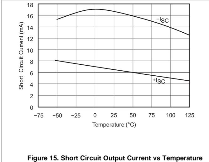
**Figure 15. Short Circuit Output Current vs Temperature**
