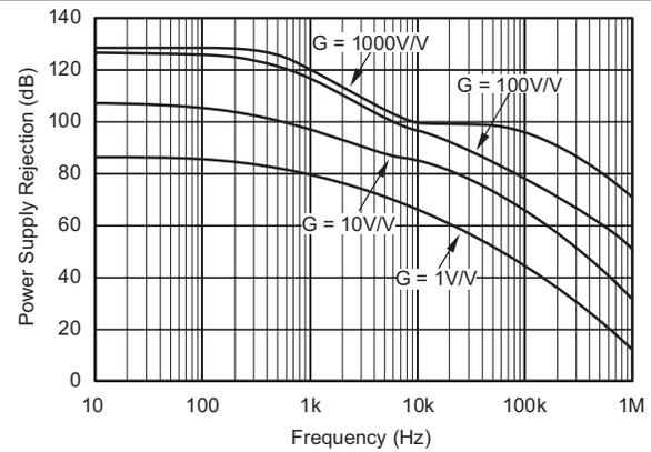
**Figure 4. Negative Power Supply Rejection vs Frequency**
