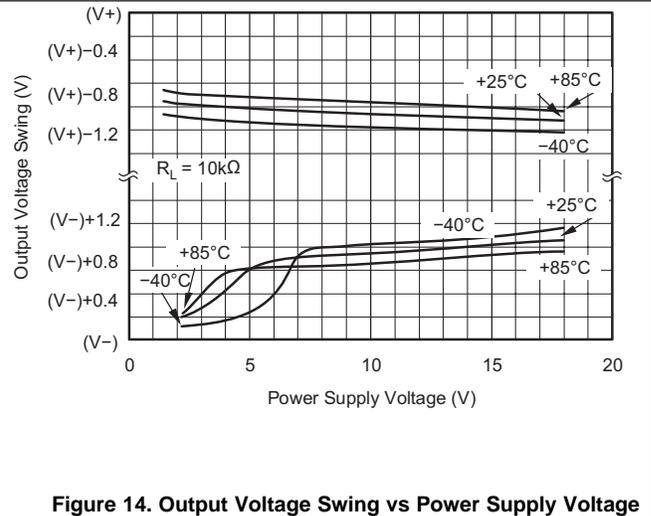
**Figure 14. Output Voltage Swing vs Power Supply Voltage**
