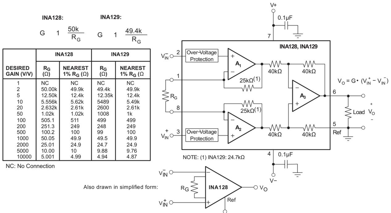
**Figure 24. Basic Connections**
