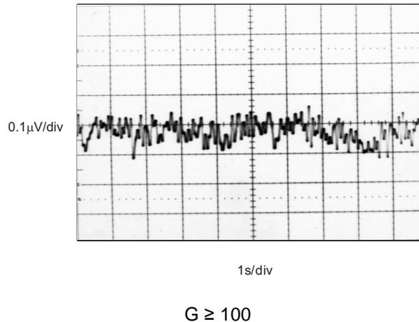
**Figure 23. 0.1-Hz to 10-Hz Input-Referred Voltage Noise**
