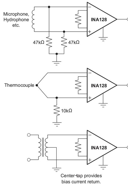
**Figure 26. Providing an Input Common-Mode Current Path**
