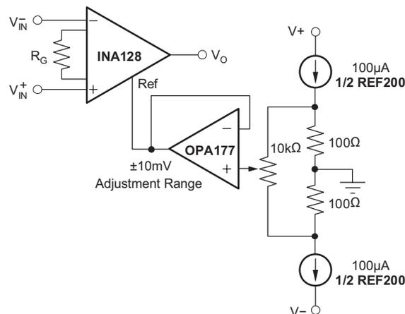
**Figure 25. Optional Trimming of Output Offset Voltage**
