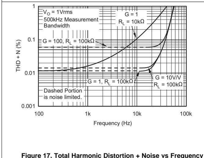
**Figure 17. Total Harmonic Distortion + Noise vs Frequency**
