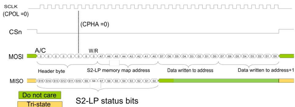
Figure 28. SPI read sequence
