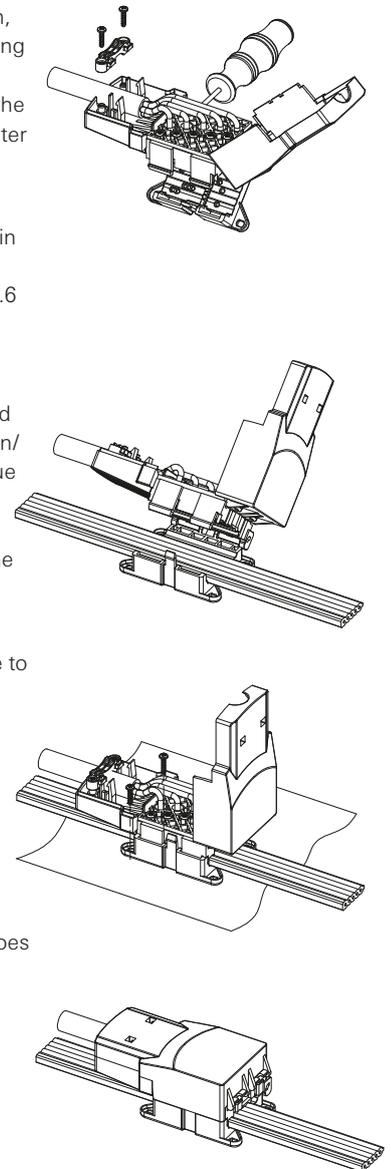
Sheath strip length 2-pole feed: 25 mm
