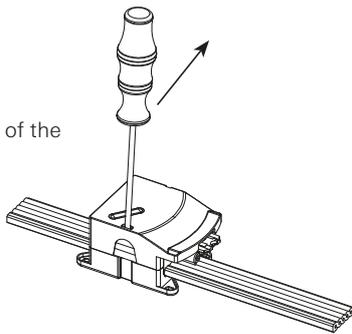
3. Loosen the contact screws.
