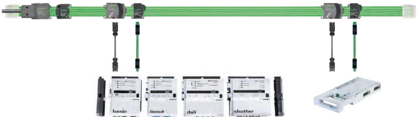
The 7-pole **gesis**®NRG BASIC+SELV flat cable 5G2.5+2x1.5 mm<sup>2</sup> supplies energy (3-phase) and the KNX to the area. Consumers/field devices/actuators/module units can then be supplied directly with mains power via 3-pole flat cable adapters with phase selection; the KNX is tapped via a further 2-pole adapter. With the use of Wieland KNX systems, the room automation components are then connected via a **gesis**® connecting cable.
