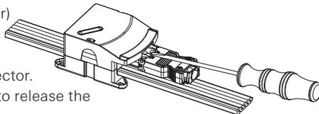
2. Push interlock in the direction of the arrow and open the cover.
