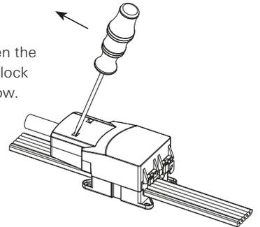
2. Loosen the contact screws and connection screws.
