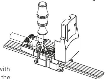
3. Unlock the baseplate interlock with a tool (screwdriver) and remove the module from the flat cable.
