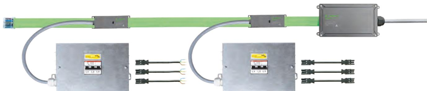
The 5-pole **gesis**® NRG flat cable 5G10 mm<sup>2</sup> supplies energy (3-phase, up to 50 A) to the area. Here, **gesis**® RAN system distribution units are then connected to pre-assembled connection cables and flat cable adapters. The system distribution units are built to the customer's wishes and contain the necessary protective devices as well as the pluggable outlets needed for the application.
