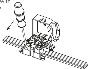
5. Close the contact openings in the cable with a cable repair patch.
