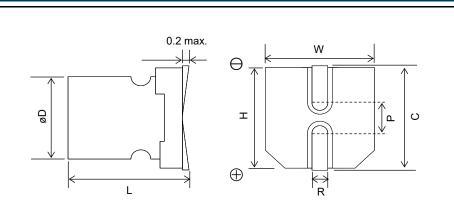
Unit : mm Size L +0.1 -0.4 P\*1 W±0.2 øD±0.5 H±0.2 C±0.2 R code 4.0 4.3 5.0 0.6 to 0.8 Α5 5.4 4.3 1.0 B6 5.0 5.9 5.3 5.3 6.0 0.6 to 0.8 1.4 C6 6.3 5.9 6.6 6.6 7.3 0.6 to 0.8 2.1 **E**7 8.0 6.9 8.3 8.3 9.0 0.6 to 0.8 3.2 F8 10.0 7.9 10.3 10.3 11.0 0.6 to 0.8 4.6
