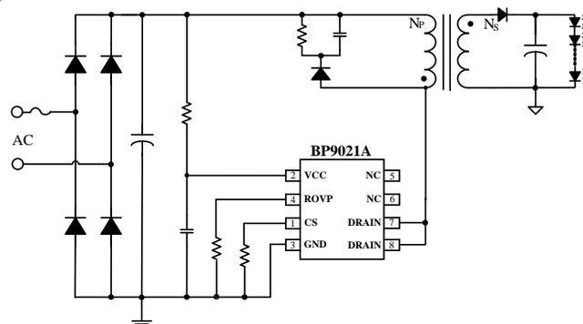
Figure 1. Typical application circuit for BP9021A
