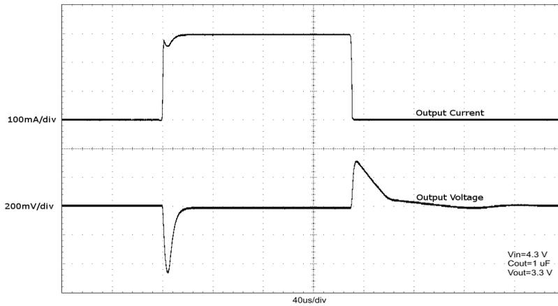
Figure 17. Load Transient Response ( $1.0\ \mu\text{F}$ )
