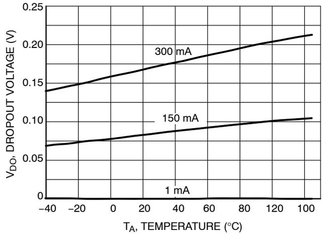
Figure 4. Dropout Voltage vs. Temperature (Over Current Range)
