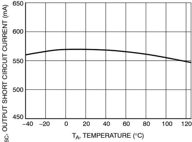
Figure 10. Output Short Circuit Current vs. Temperature
