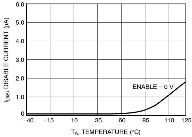
**Figure 7. Ground Current (Sleep Mode) vs. Temperature**
