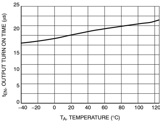
Figure 14. Output Turn On Time vs. Temperature
