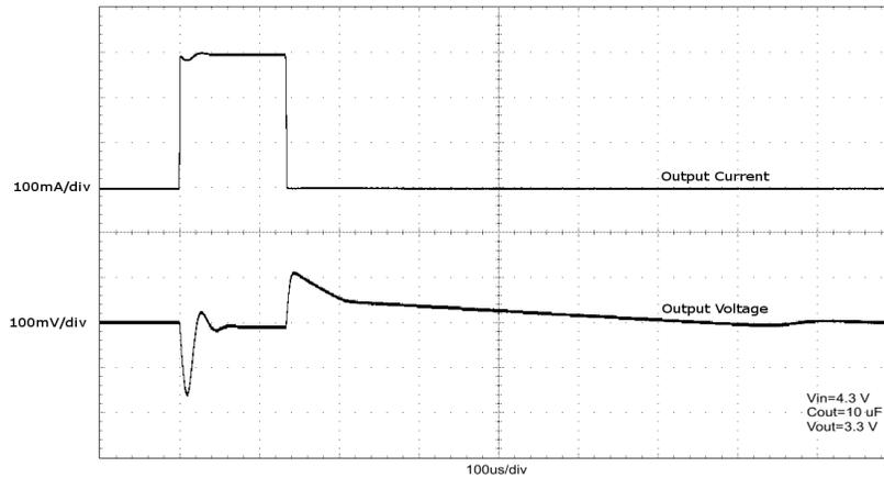
Figure 18. Load Transient Response ( $10\ \mu\text{F}$ )
