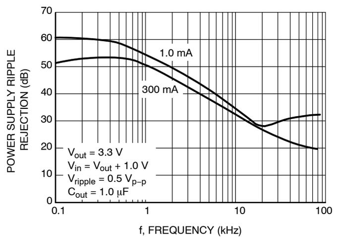
Figure 15. Power Supply Ripple Rejection vs. Frequency
