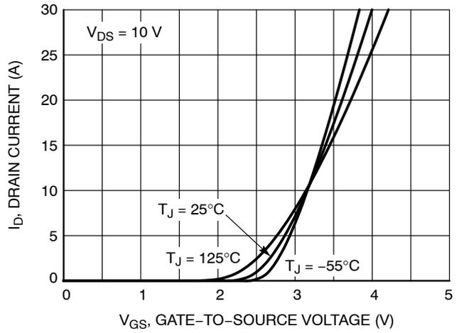
Figure 2. Transfer Characteristics
