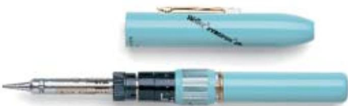
Manual ignited lightweight Butane gas operated soldering iron with solder, hot blow and blow torch functions. Supplied with aluminium protective cap with pocket clip and safety feature to prevent the cap being fitted when the iron is on. Temperature variable between 400°C to 500°C when used as a soldering iron, up to 650°C when used as a hot air blower and 1300°C when used as a blow torch.
