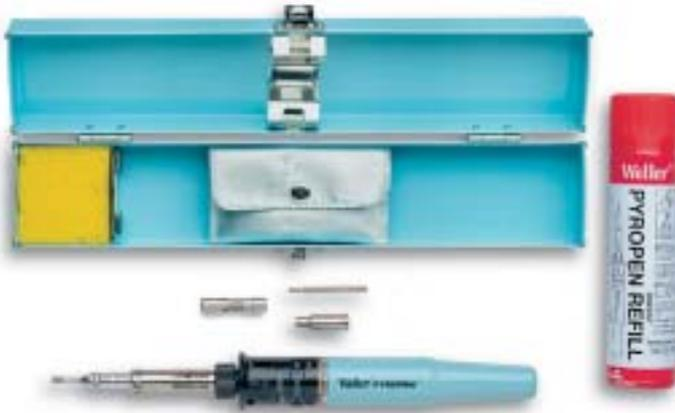
Manually ignited butane gas operated, soldering iron with solder, hot blow and blow torch functions. The tool has a rapid heat up time and duration of operation from one filling of approx. 3 hours. It is temperature variable between 350°C to 500°C when used as a soldering iron and up to 650°C when used as a hot air blower and 1300°C when used as a blow torch.
