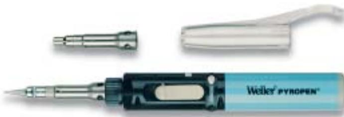
Butane gas operated self igniting soldering iron with solder and hot blow functions. Temperature variable up to 500°C. The tool has a rapid heat up and a duration of approx. 1 hour. Supplied with a protective cap with a safety feature to switch off the iron .
