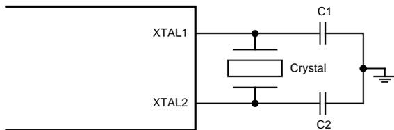
(3) Crystal Oscillator( Ceramic resonator): 4MHz(2MHz) - 16.6MHz
