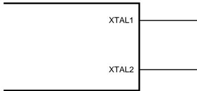
(2) Crystal Oscillator 32.768kHz and internal RC: 16.6MHz
