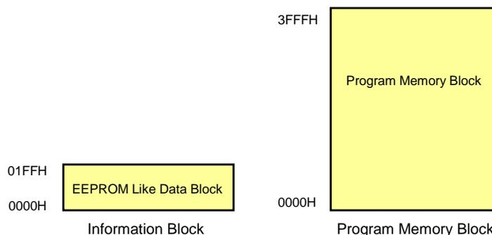
The SH79F1612B embeds 16K flash program memory for program code. The flash program memory provides electrical erasure and programming and supports In-Circuit Programming (ICP) mode and Self-Sector Programming (SSP) mode. 1024 bytes per sector.
