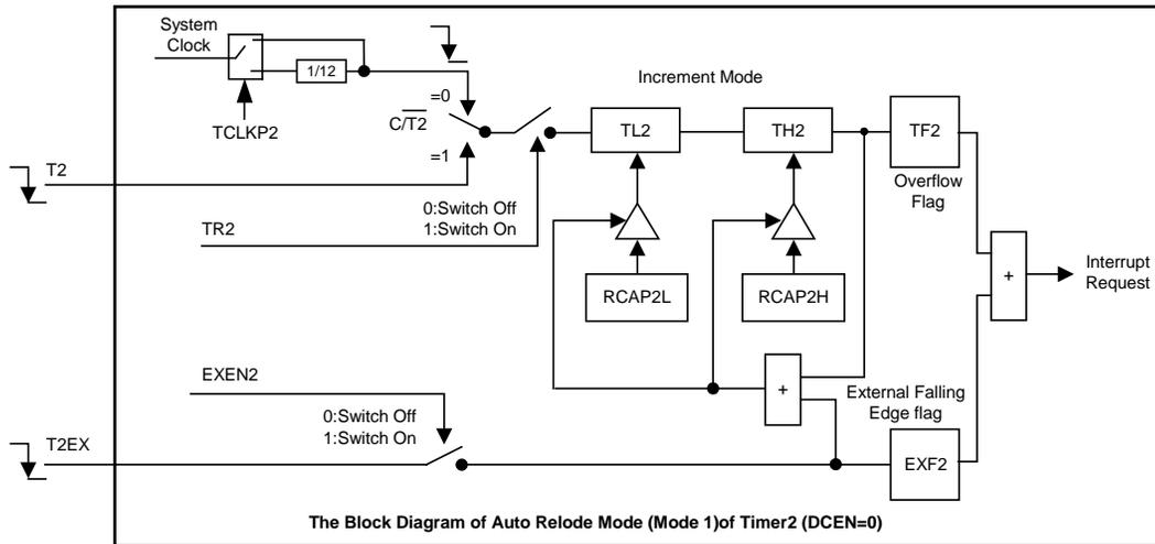
Setting the DCEN bit enables Timer2 to count up or down. When DCEN = 1, the T2EX pin controls the direction of the count, and EXEN2's control is invalid.
