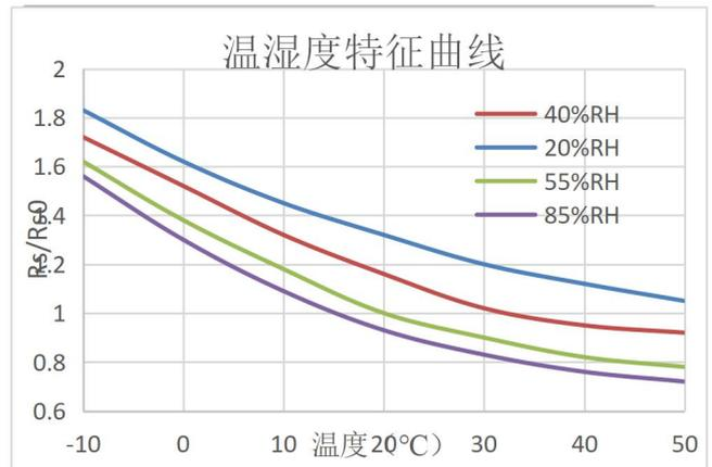
**Fig4. Typical temperature/humidity characteristics**
