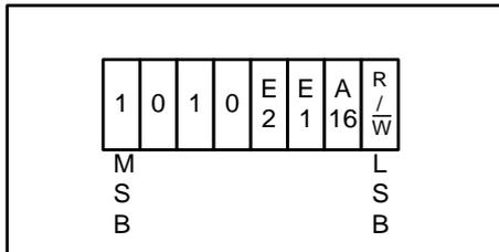
The two E2 and E1 device address bits allow as many as four devices on the same bus. These bits must compare to their corresponding hardwired input pins.
