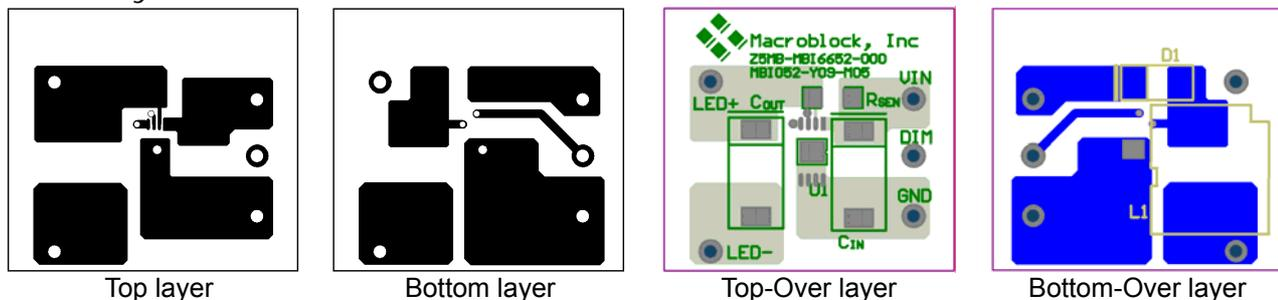
Figure 65. The layout diagram of the MBI6652 GMS
