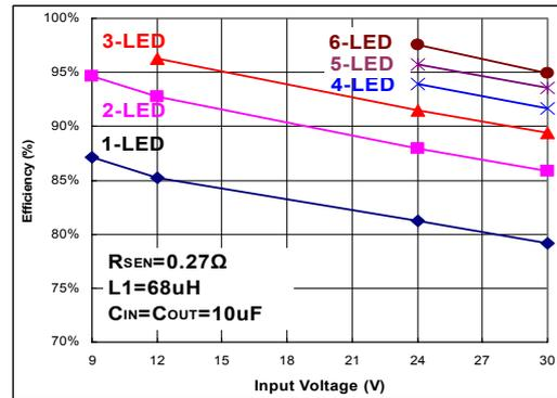
Fig 7.  $I_{OUT}=370\text{ mA}$
