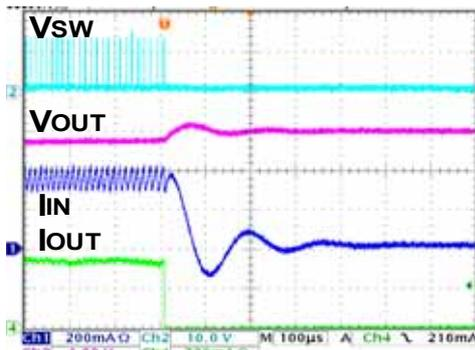
Figure 61. Open-circuit protection
