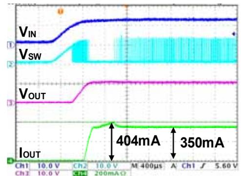
Figure 58. The start-up waveform @  $V_{IN}=12V, V_{OUT}= 10.8, R_{SEN}=0.27$
