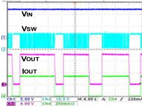
Figure 63. Thermal protection
