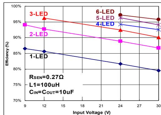
Fig 9.  $I_{OUT}=370\text{ mA}$
