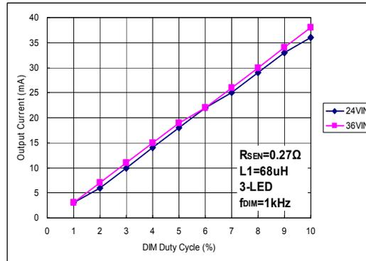
Figure 60. DIM duty cycle: 1% ~ 10%
