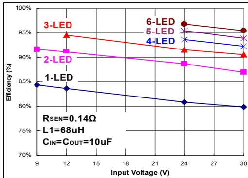
Fig 6.  $I_{OUT}=715\text{ mA}$
