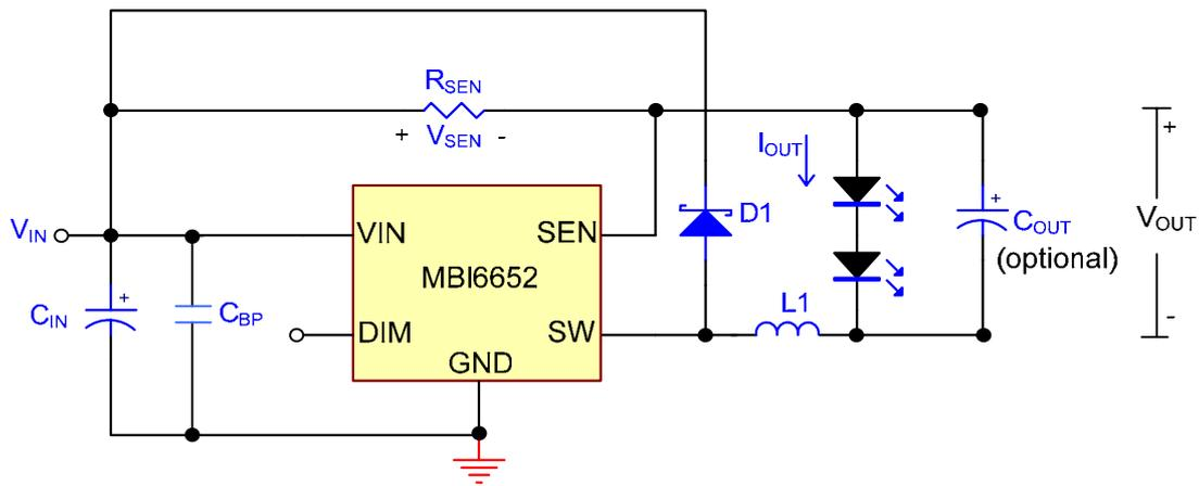
$C_{IN}$ : VISHAY, 293D106X9050D2TE3, D case Tantalum Capacitor
