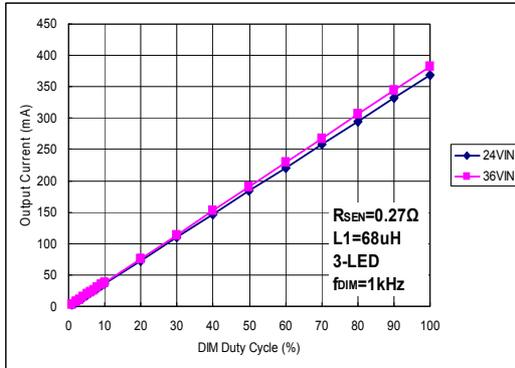
Figure 59. DIM duty cycle: 1% ~ 100%
