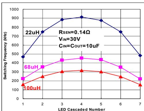
Fig 44.  $I_{OUT}=715\text{ mA}$
