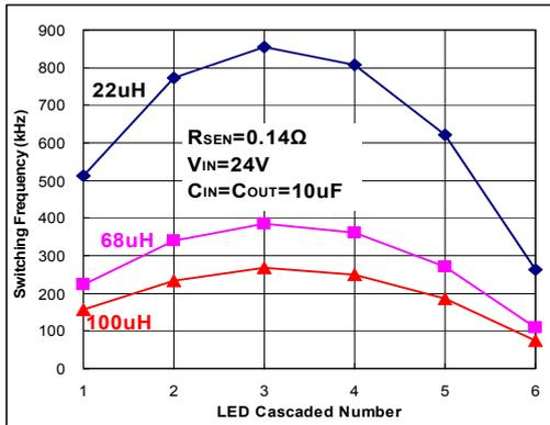
Fig 42.  $I_{OUT}=715\text{ mA}$
