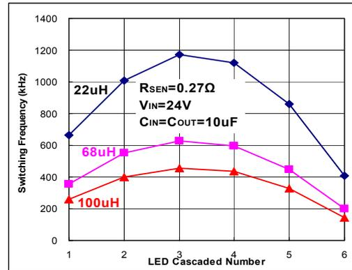
Fig 43.  $I_{OUT}=370\text{ mA}$
