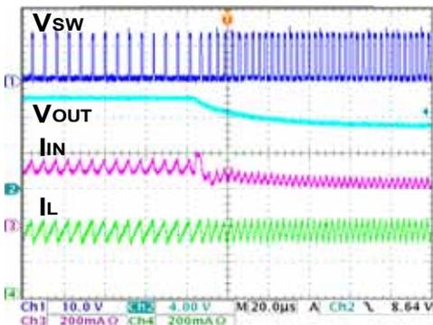
Figure 62. Short-circuit protection
