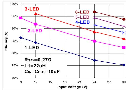
Fig 5.  $I_{OUT}=370\text{ mA}$
