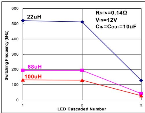
Fig 40.  $I_{OUT}=715\text{ mA}$
