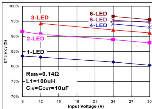
Fig 8.  $I_{OUT}=715\text{ mA}$
