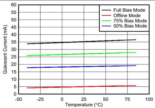
Figure 7-22. Supply Current vs Temperature
