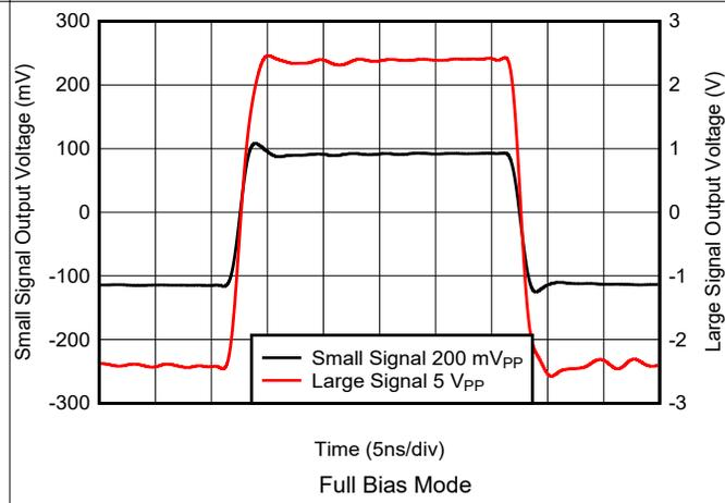
**Figure 7-4. Small-Signal and Large-Signal Pulse Responses**
