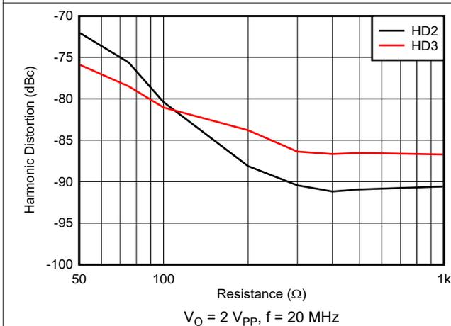
Figure 7-11. Harmonic Distortion vs Load Resistance
