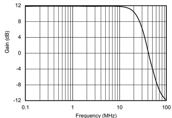
Figure 9-2. Buffered Single-Supply Active Filter: Gain vs Frequency
