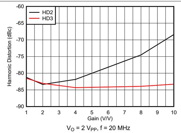
Figure 7-12. Harmonic Distortion vs Noninverting Gain
