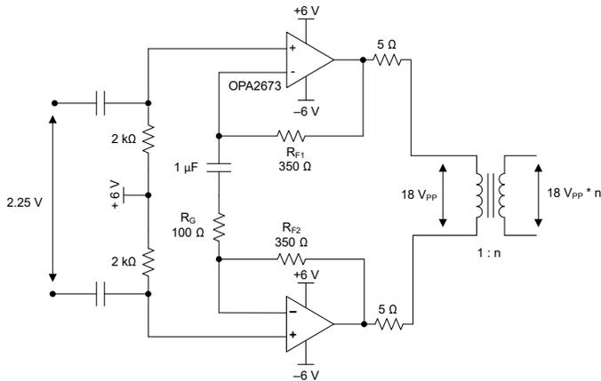
Figure 9-3. Typical Schematic for PLC Applications
