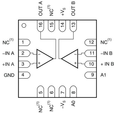
**Figure 6-1. RGV Package, 16-Pin VQFN (Top View)**
