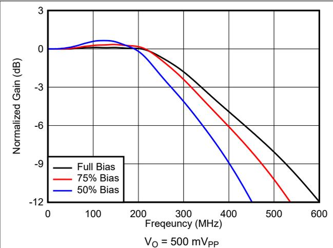
**Figure 7-2. Small-Signal Frequency Response Over Power Settings**
