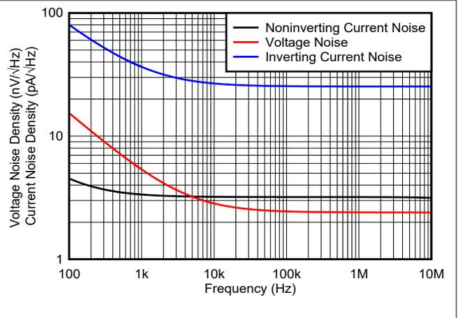
Figure 7-16. Input Voltage and Current Noise Density
