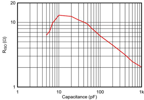
Figure 8-7. Recommended  $R_{ISO}$  vs Capacitive Load
