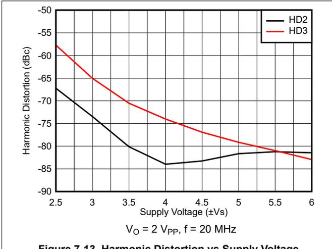
Figure 7-13. Harmonic Distortion vs Supply Voltage
