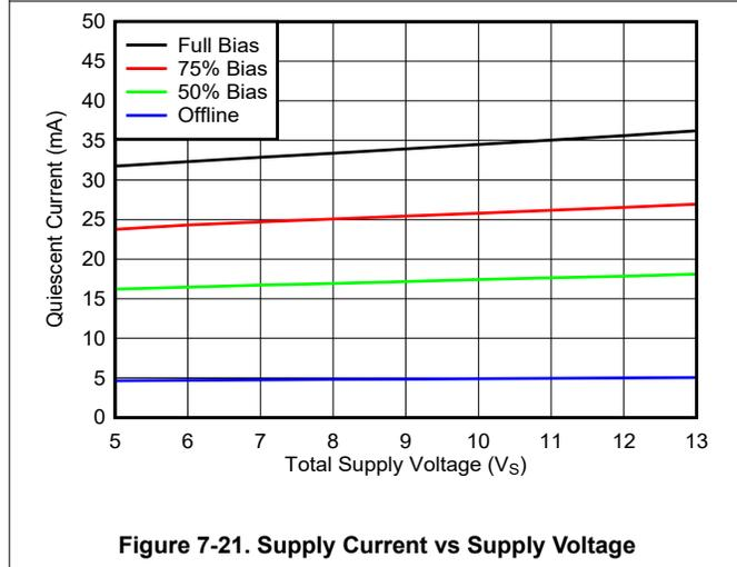
Figure 7-21. Supply Current vs Supply Voltage
