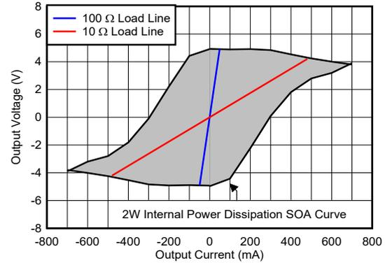
Figure 8-5. Output Voltage and Current Limitations
