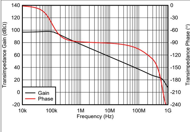
Figure 7-15. Open-Loop Transimpedance Gain and Phase
