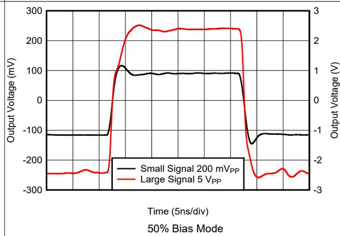
**Figure 7-6. Small-Signal and Large-Signal Pulse Responses**
