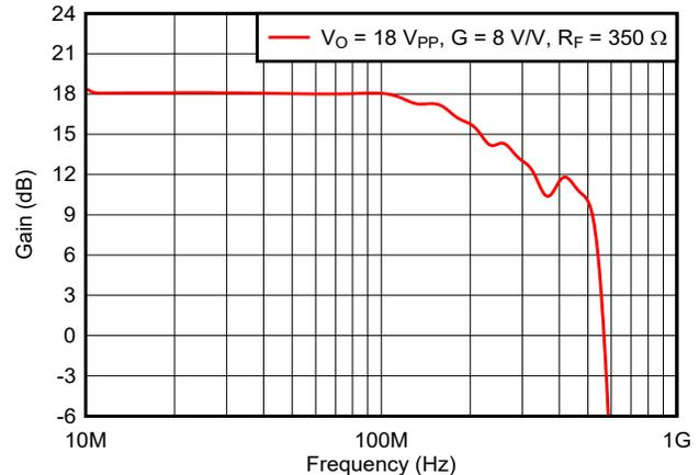
Figure 9-4. Large-Signal Frequency Response
