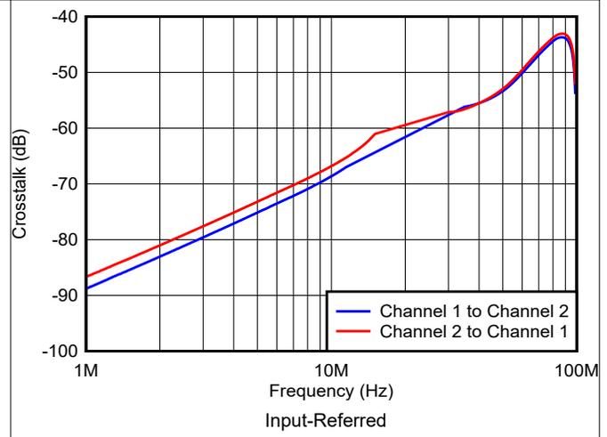
Figure 7-8. Channel-to-Channel Crosstalk
