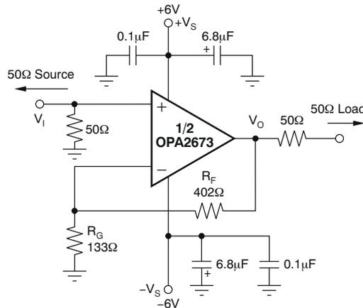
Figure 8-1. DC-Coupled, G = +4 V/V, Bipolar Supply
