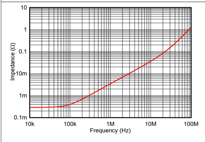
Figure 7-17. Closed-Loop Output Impedance vs Frequency
