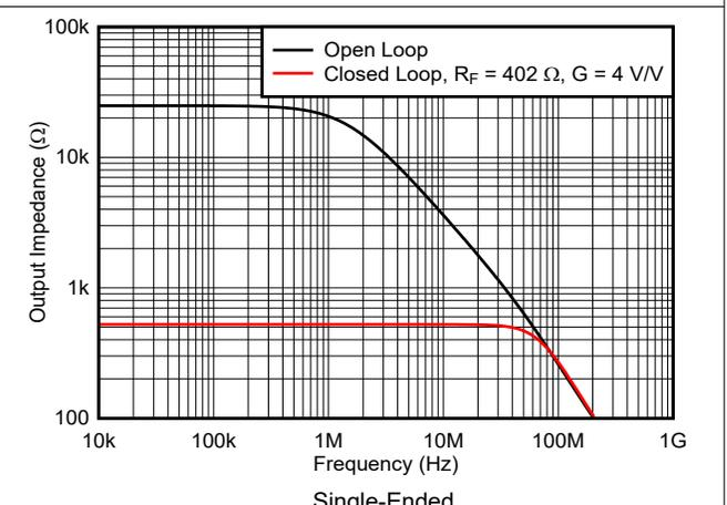
Figure 7-18. Active Off-Line Impedance vs Frequency
