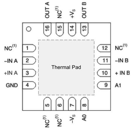
**Figure 6-2. RGV Package, 16-Pin VQFN (Bottom View)**
