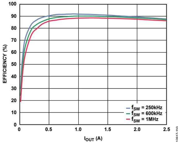
Figure 10. Channel 3/Channel 4 Efficiency Curve,  $V_{IN} = 12\text{ V}$ ,  $V_{OUT} = 1.8\text{ V}$ , FPWM Mode
