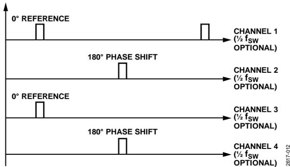
Figure 31. Phase Shift Diagram, Four Buck Regulators
