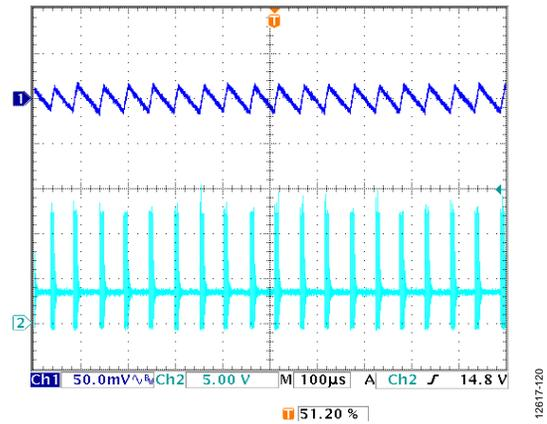
Figure 20. Steady State Waveform at Light Load,  $V_{IN} = 12\text{ V}$ ,  $V_{OUT} = 3.3\text{ V}$ ,  $I_{OUT} = 30\text{ mA}$ ,  $f_{SW} = 600\text{ kHz}$ ,  $L = 4.7\text{ }\mu\text{H}$ ,  $C_{OUT} = 47\text{ }\mu\text{F} \times 2$ , Automatic PWM/PSM Mode, Channel 1 =  $V_{OUTx}$ , Channel 2 =  $SWx$
