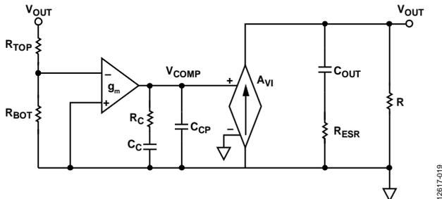
Figure 39. Simplified, Peak Current-Mode Control, Small Signal Circuit
