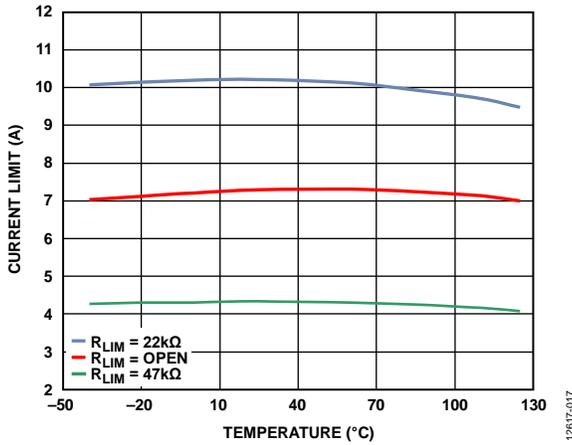
Figure 17. Channel 1/Channel 2 Current Limit vs. Temperature
