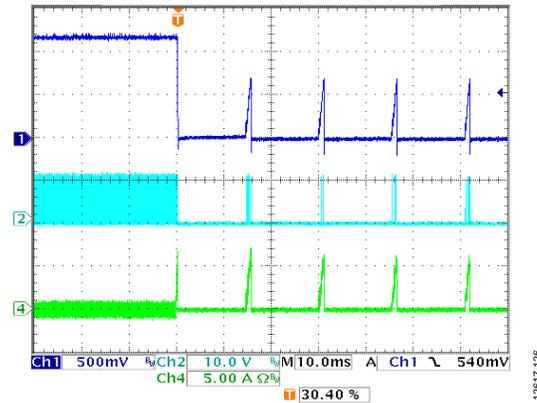
Figure 26. Short-Circuit Protection Entry,  $V_{IN} = 12\text{ V}$ ,  $V_{OUT} = 1.2\text{ V}$ ,  $f_{SW} = 600\text{ kHz}$ ,  $L = 1\text{ }\mu\text{H}$ ,  $C_{OUT} = 47\text{ }\mu\text{F} \times 2$ , Channel 1 =  $V_{OUTX}$ , Channel 2 = SWX, Channel 4 =  $I_{LX}$
