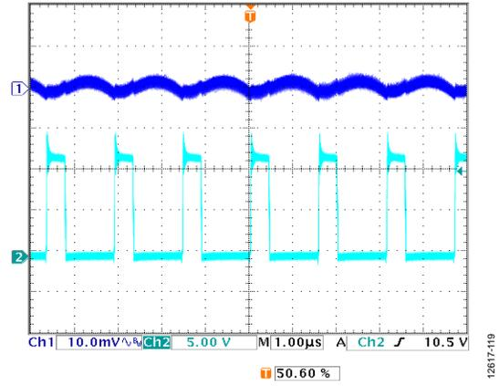
Figure 19. Steady State Waveform at Heavy Load,  $V_{IN} = 12\text{ V}$ ,  $V_{OUT} = 3.3\text{ V}$ ,  $I_{OUT} = 3\text{ A}$ ,  $f_{SW} = 600\text{ kHz}$ ,  $L = 4.7\text{ }\mu\text{H}$ ,  $C_{OUT} = 47\text{ }\mu\text{F} \times 2$ , FPWM Mode, Channel 1 =  $V_{OUTx}$ , Channel 2 =  $SWx$
