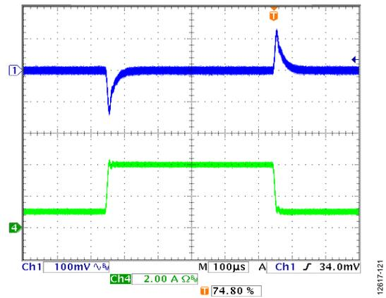
Figure 21. Channel 1/Channel 2 Load Transient, 1 A to 4 A,  $V_{IN} = 12\text{ V}$ ,  $V_{OUT} = 3.3\text{ V}$ ,  $f_{SW} = 600\text{ kHz}$ ,  $L = 2.2\text{ }\mu\text{H}$ ,  $C_{OUT} = 47\text{ }\mu\text{F} \times 2$ , Channel 1 =  $V_{OUTx}$ , Channel 4 =  $I_{OUTx}$
