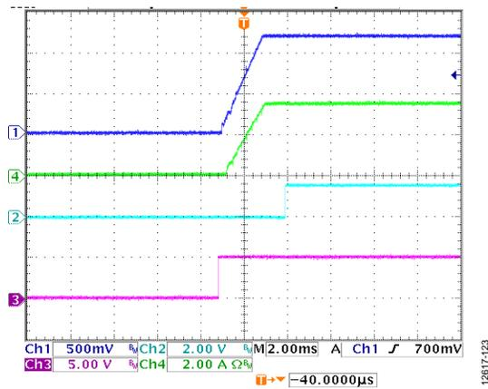
Figure 23. Channel 1 Soft Start with 4 A Resistance Load,  $V_{IN} = 12\text{ V}$ ,  $V_{OUT} = 1.2\text{ V}$ ,  $f_{SW} = 600\text{ kHz}$ ,  $L = 1\text{ }\mu\text{H}$ ,  $C_{OUT} = 47\text{ }\mu\text{F} \times 2$ , Channel 1 =  $V_{OUT1}$ , Channel 2 = PWRGD, Channel 3 = EN1, Channel 4 =  $I_{OUT1}$
