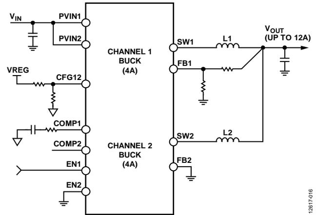
Figure 35. Parallel Operation for Channel 1 and Channel 2
