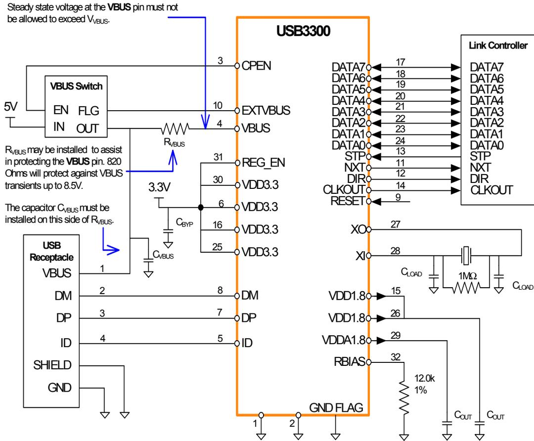
Figure 6 USB3300 Application Diagram (Host or OTG)
