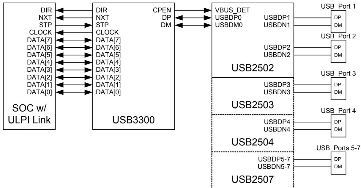
**Figure 8 Expanding Downstream Ports for USB3300 Host Applications**
