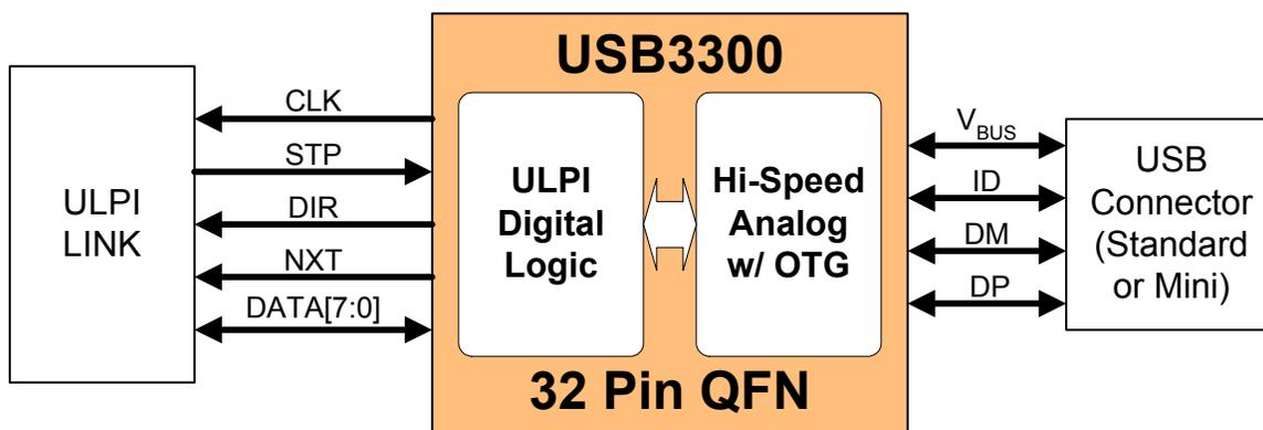
**Figure 1 Basic ULPI USB Device Block Diagram**
