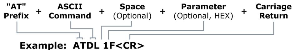
To read a parameter value stored in the RF modem’s register, omit the parameter field.
