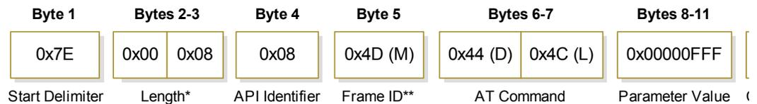
\* Length [Bytes] = API Identifier + Frame ID + AT Command + Parameter Value
