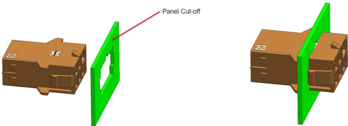
**5.1.4 Insert the TPA into receptacle or plug mentioned in the SD.**
