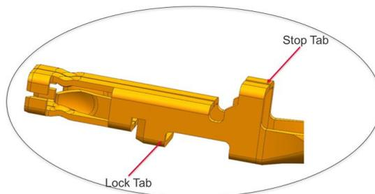
**5.1.2 Insert the recommended Male crimp terminals as in the SD into the Plug housing.** Terminals are inserted in the opposite orientation for both top and bottom row.
