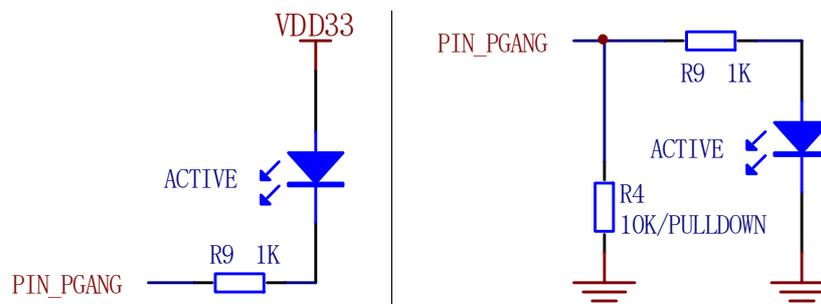
The statically driven PGANG pin can be used to control power to external devices, such as powering off peripherals during Suspend.
