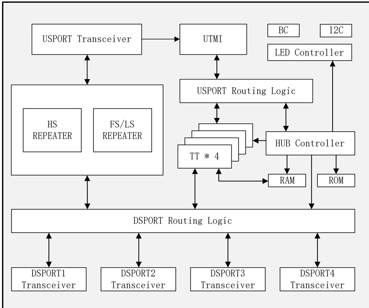
Figure 2-1 is a block diagram of the internal structure of the HUB controller system. The HUB controller consists of three main modules: Repeater, TT and controller. The controller is similar to an MCU processor for global management and control. The routing logic will connect the port to Repeater when the speed of uplink port and downlink port are the same, and connect the port to TT when the speed of uplink port and downlink port are not the same.
