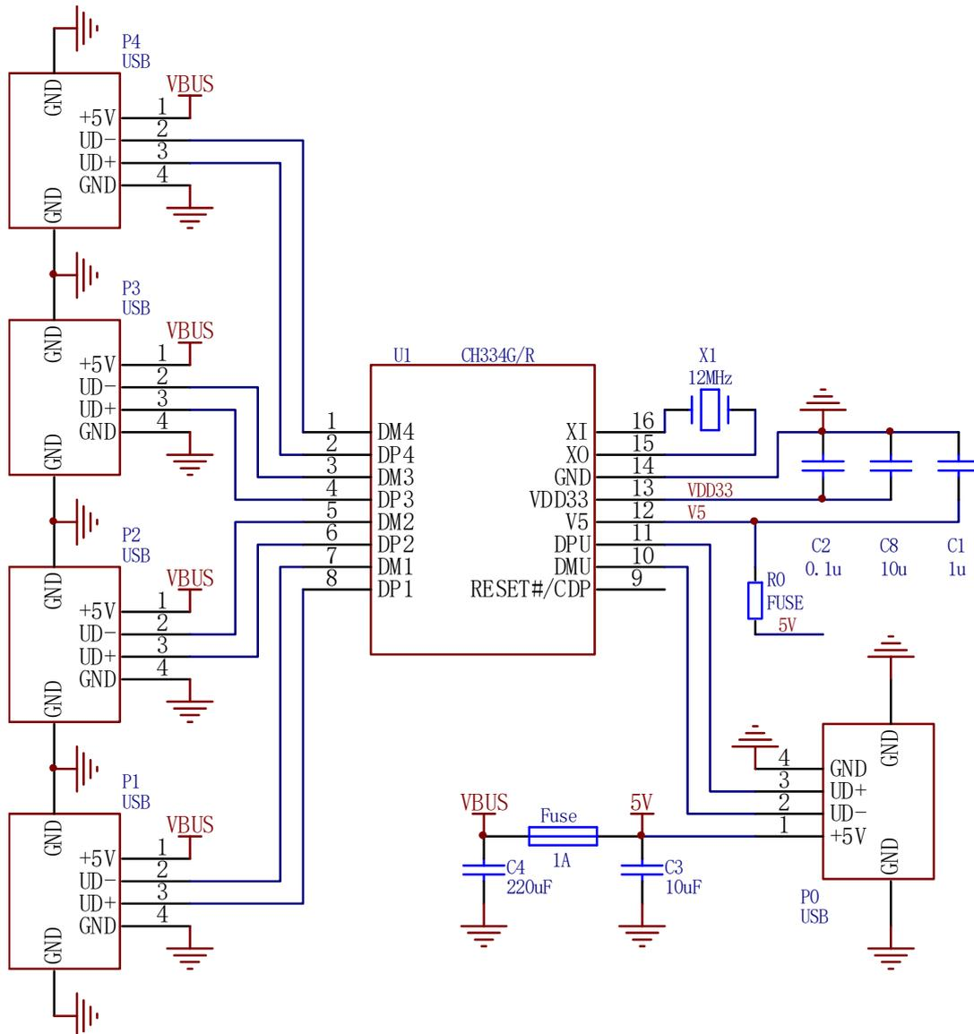
R0 is a 100mA fuse resistor, for simplified applications,  $0\Omega$  can be used. if there is an overvoltage protection device, it is connected to pin V5.
