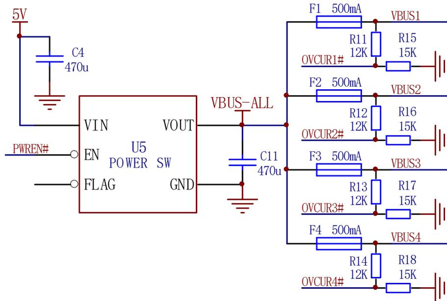
Figure 3-1-2 is another option, U5 is the shared power switch chip, F1 to F4 are the insurance resistors, and C11 is selected as needed. Alternatively, there is a simplified application that removes power control, based on Figure 3-1-2 that omits U5/C4 and shorts the VBUS-ALL to 5V.
