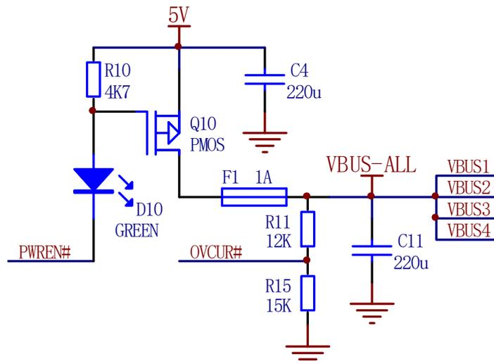
Figure 3-1-4 is a simplified schematic, for principle reference only. The default configuration  $OC\_LEVEL=0$ , R11 and R15 voltage divider to select the overcurrent detection point for VBUS down to about 4V. If the configuration  $OC\_LEVEL = 1$ , then you can remove R15 and change R11 to 1K.
