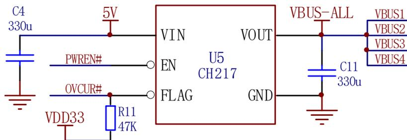
U5 is a USB current-limiting power switch chip. R11 can be omitted in the default configuration, and the capacity of C11 can be selected as needed.
