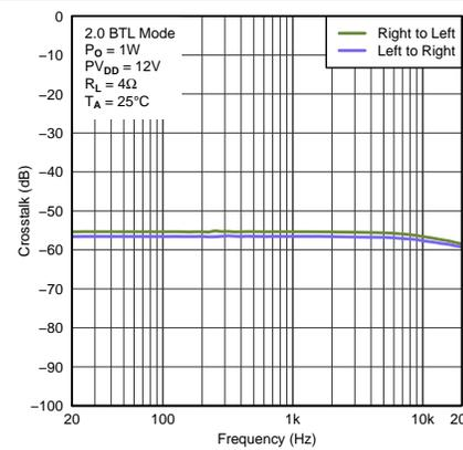
Figure 28. Crosstalk vs Frequency
