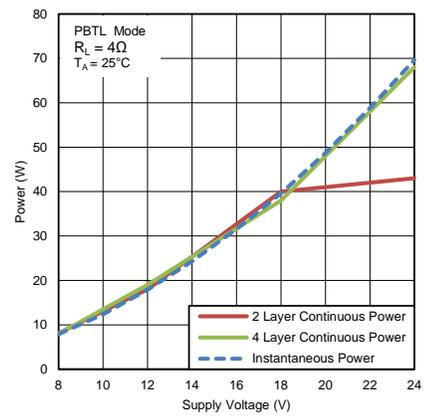
Figure 42. Power vs Supply Voltage (PBTL Mode)
