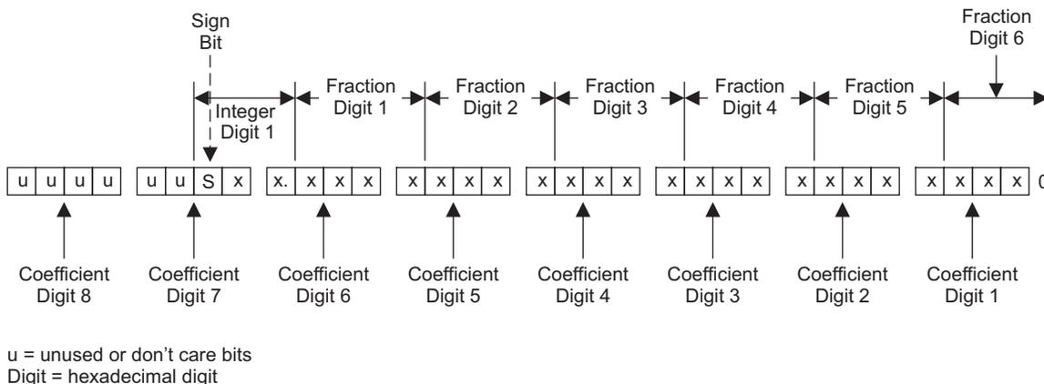
Figure 66. Alignment of 3.23 Coefficient in 32-Bit I<sup>2</sup>C Word
