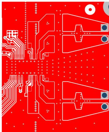
**Figure 71. Layout Example (Stereo) - Top Layer**
