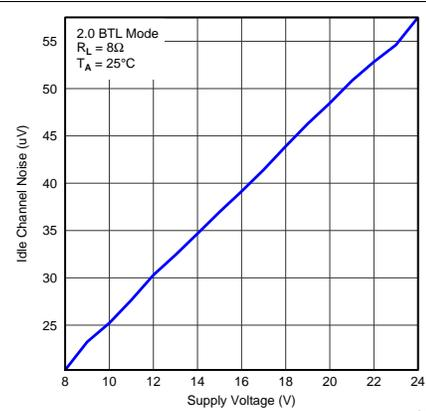
Figure 6. Idle Channel Noise vs Supply Voltage
