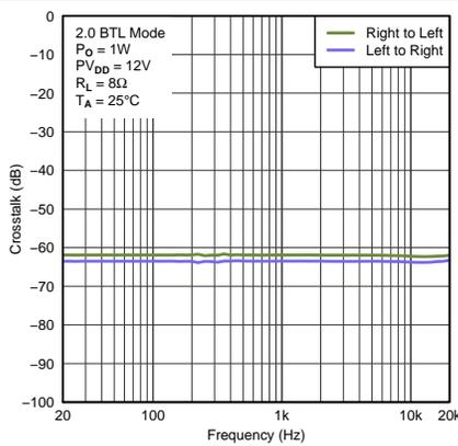
Figure 27. Crosstalk vs Frequency
