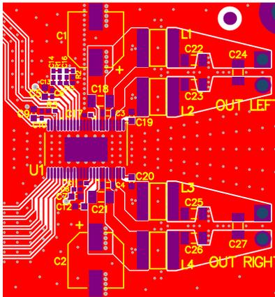
**Figure 70. Layout Example (Stereo) - Top View Composite**
