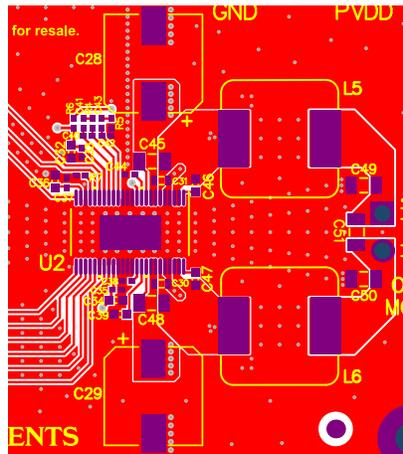
Figure 73. Layout Example (Mono) - Top View Composite
