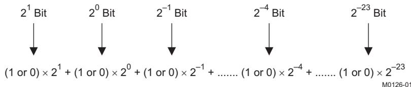
Figure 65. Conversion Weighting Factors—3.23 Format to Floating Point
