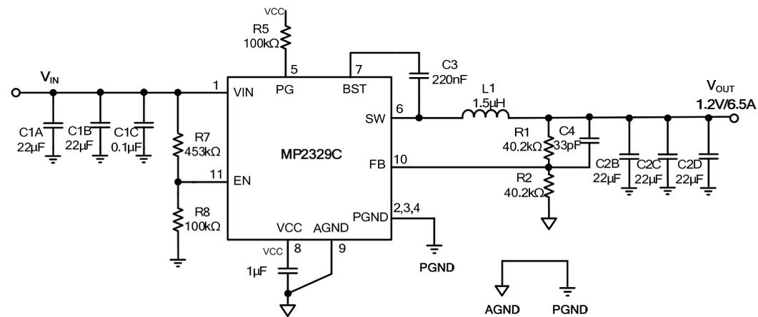
**Figure 14:  $V_{IN} = 19V$ ,  $V_{OUT} = 1.2V/6.5A$**
