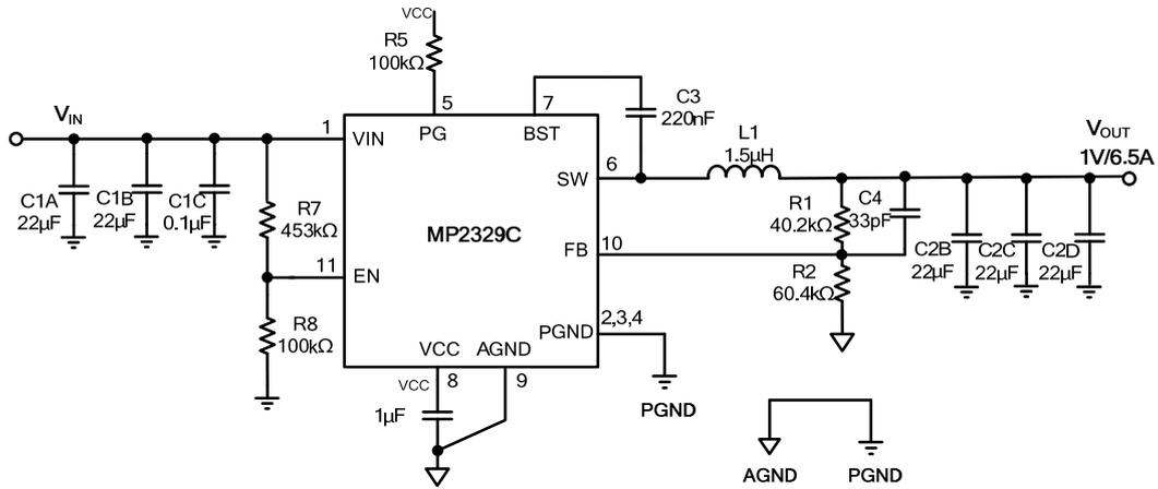
**Figure 15:  $V_{IN} = 19V$ ,  $V_{OUT} = 1V/6.5A$**
