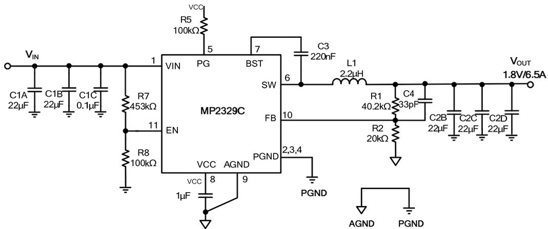
**Figure 12:  $V_{IN} = 19V$ ,  $V_{OUT} = 1.8V/6.5A$**
