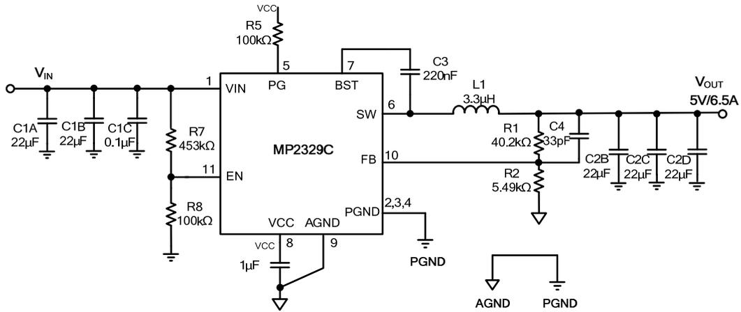
**Figure 9:  $V_{IN} = 19V$ ,  $V_{OUT} = 5V/6.5A$**
