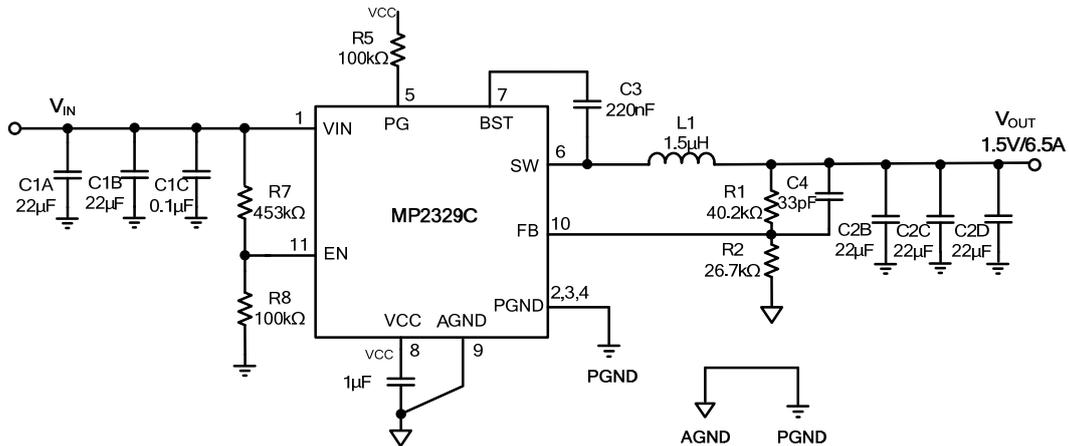
**Figure 13:  $V_{IN} = 19V$ ,  $V_{OUT} = 1.5V/6.5A$**
