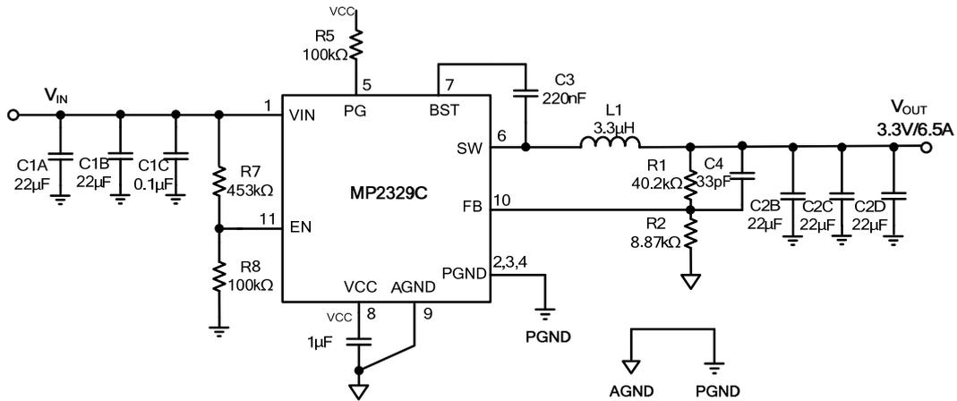
**Figure 10:  $V_{IN} = 19V$ ,  $V_{OUT} = 3.3V/6.5A$**
