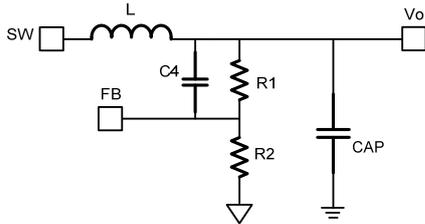
**Figure 6: Simplified Circuit without an External Ramp**
