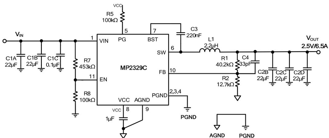
**Figure 11:  $V_{IN} = 19V$ ,  $V_{OUT} = 2.5V/6.5A$**
