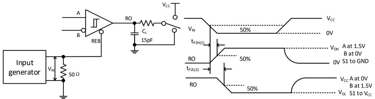
Figure 8-8. Receiver Enable Times With Driver Disabled
