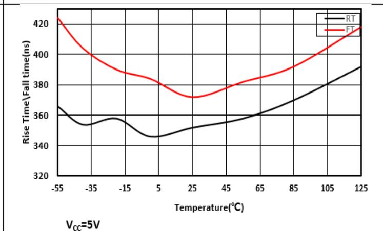
Figure 7-13 Driver Output Rise Time\Fall Time vs. Temperature
