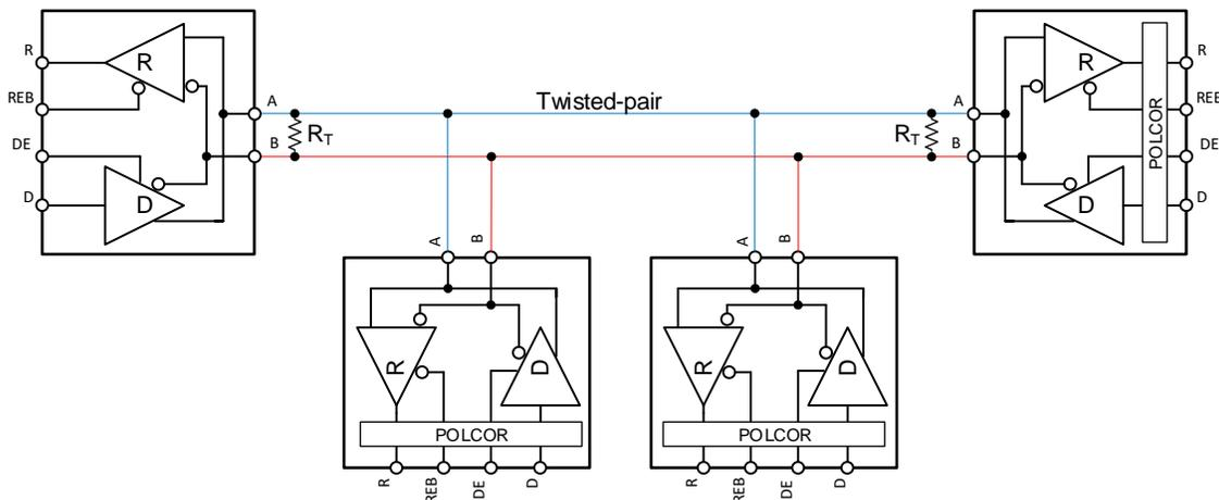
Figure 10-1. Typical RS-485 Network With CA-IF48xxHS/HM/HD Half-Duplex Transceivers
