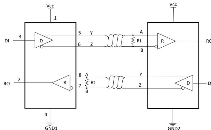
Figure 10-2. Typical RS-485 Network With CA-IF48xxFS/FM/FD Full-Duplex Transceivers
