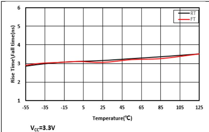
Figure 7-16 Driver Output Rise Time\Fall Time vs. Temperature
