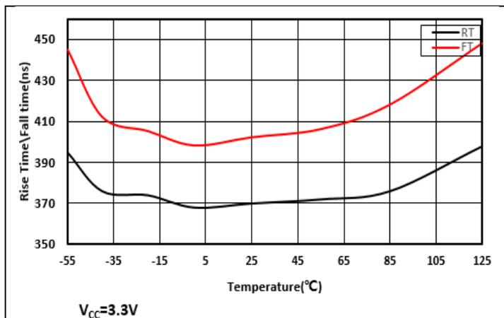
Figure 7-10 Driver Output Rise Time/Fall Time vs. Temperature
