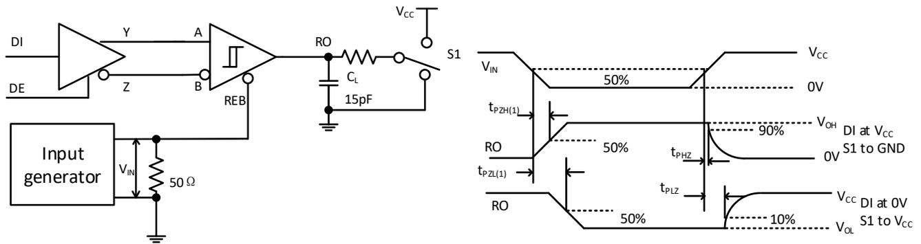
Figure 8-7. Receiver Enable/Disable Times With Driver Enabled
