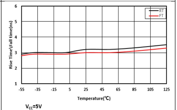
Figure 7-19 Driver Output Rise Time\Fall Time vs. Temperature
