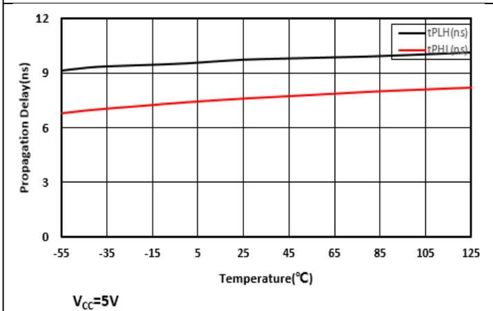
Figure 7-20 Driver Propagation Delay vs. Temperature
