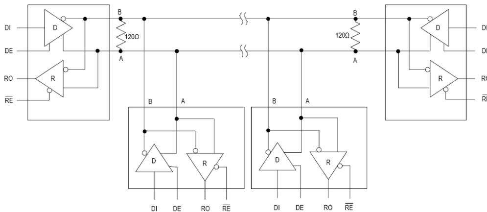
Figure 10-2. Typical isolated half-duplex RS-485 application circuit
