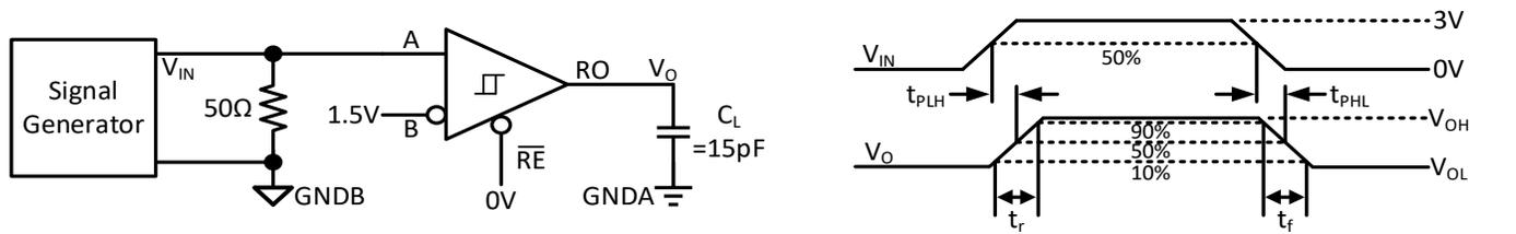
Figure 8-4. Receiver Propagation Delays
