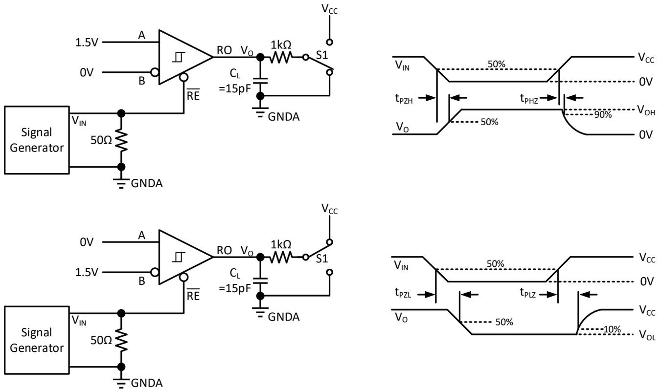
Figure 8-5. Receiver Enable and Disable Times
