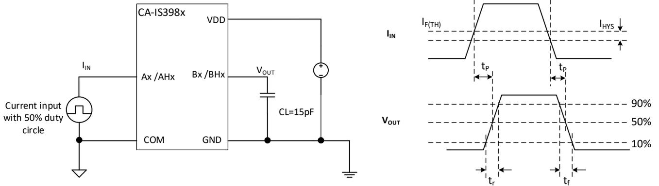
**Figure 8-1. Switching Characteristics Test Circuit and Waveform**
