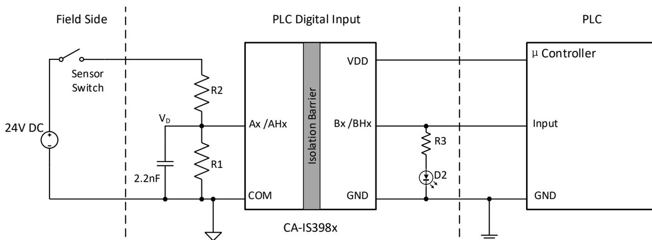
**Figure 10-2. Typical Application Circuit with Sinking Inputs**
