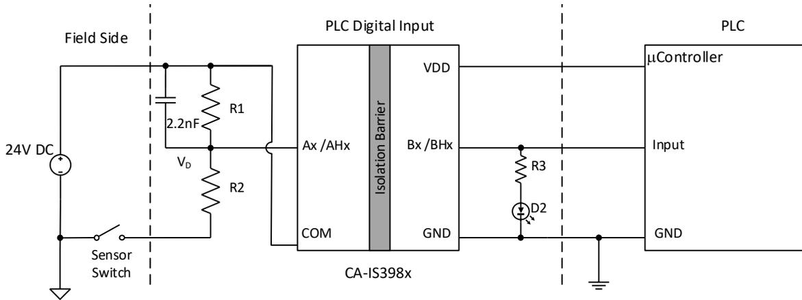
Figure 10-3. Typical Application Circuit with Sourcing Inputs
