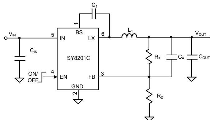
Figure 1. Schematic Diagram
