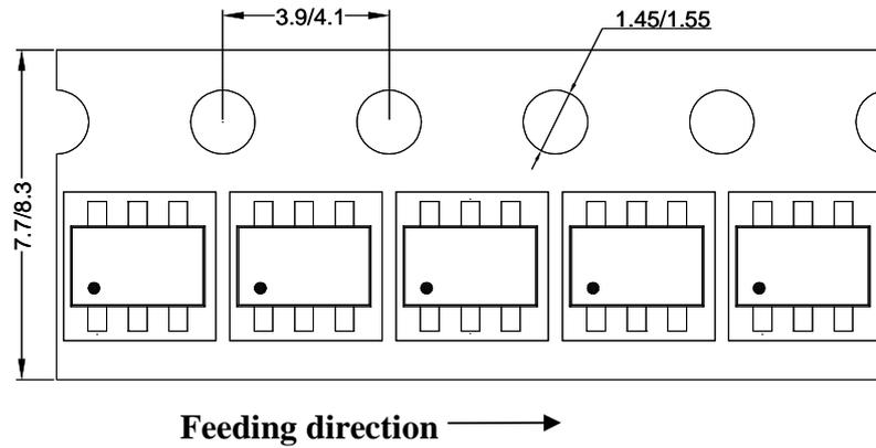
**2. Carrier Tape & Reel specification for packages**
