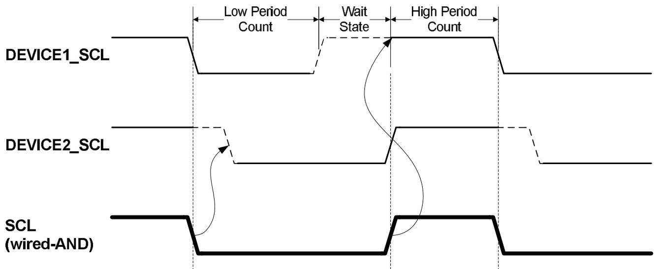
A high to low transition on the SCL line will force the line low for all masters on the bus and they start timing their low clock period. The timing length of the low clock period can vary between the masters. When a master (DEVICE1 in this
