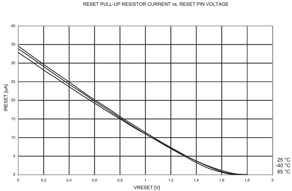
Figure 21-22. Reset Pull-up Resistor Current vs. Reset Pin Voltage ( $V_{CC} = 2.7V$ )
