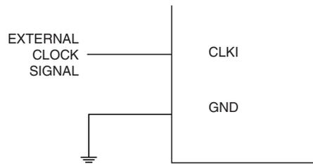
When applying an external clock, it is required to avoid sudden changes in the applied clock frequency to ensure stable operation of the MCU. A variation in frequency of more than 2% from one clock cycle to the next can lead to unpredictable behavior. It is required to ensure that the MCU is kept in reset during such changes in the clock frequency.
