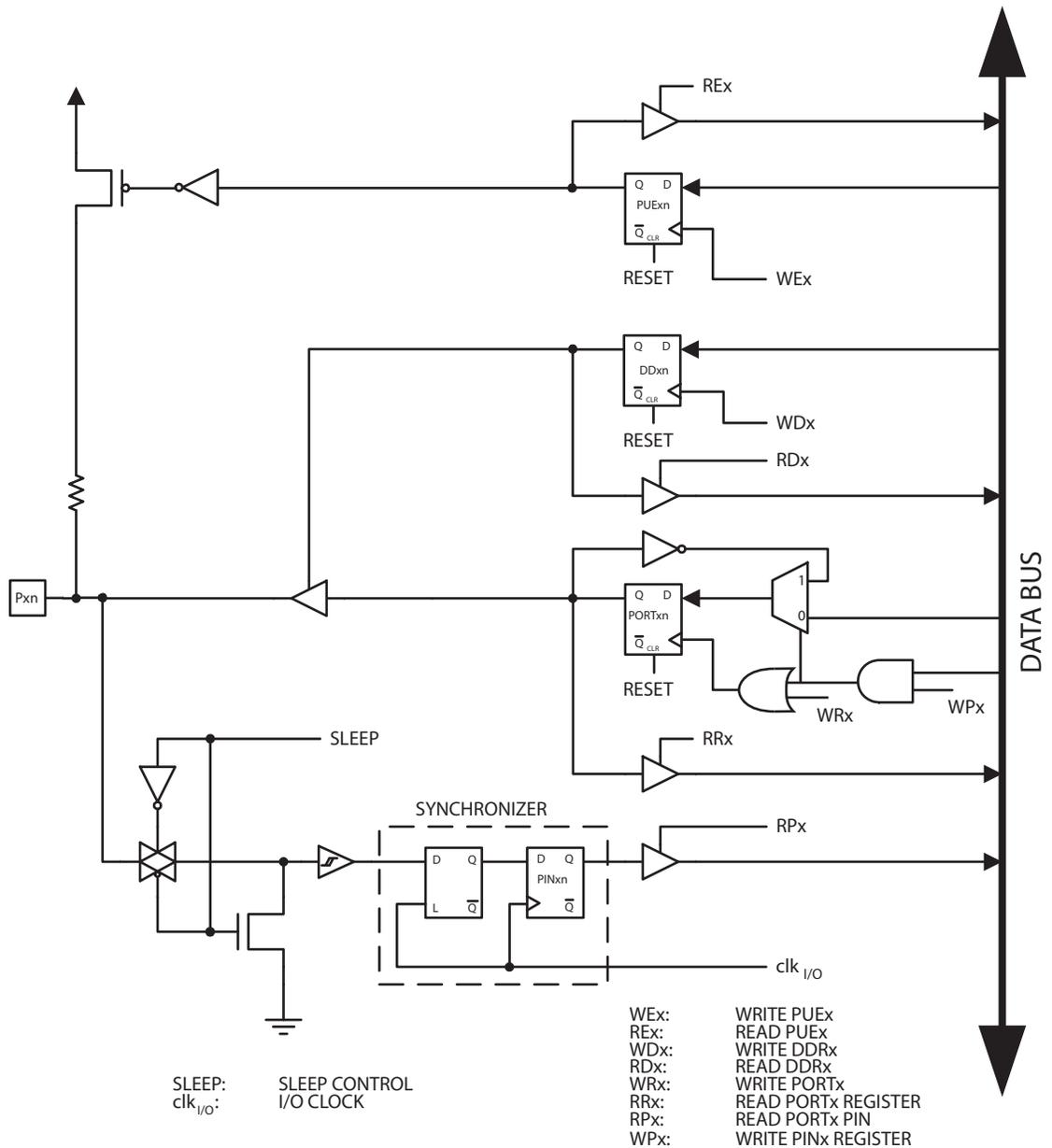
Note: 1. WEx, WRx, WPx, WDx, REx, RRx, RPx, and RDx are common to all pins within the same port. clk<sub>I/O</sub>, and SLEEP are common to all ports.
