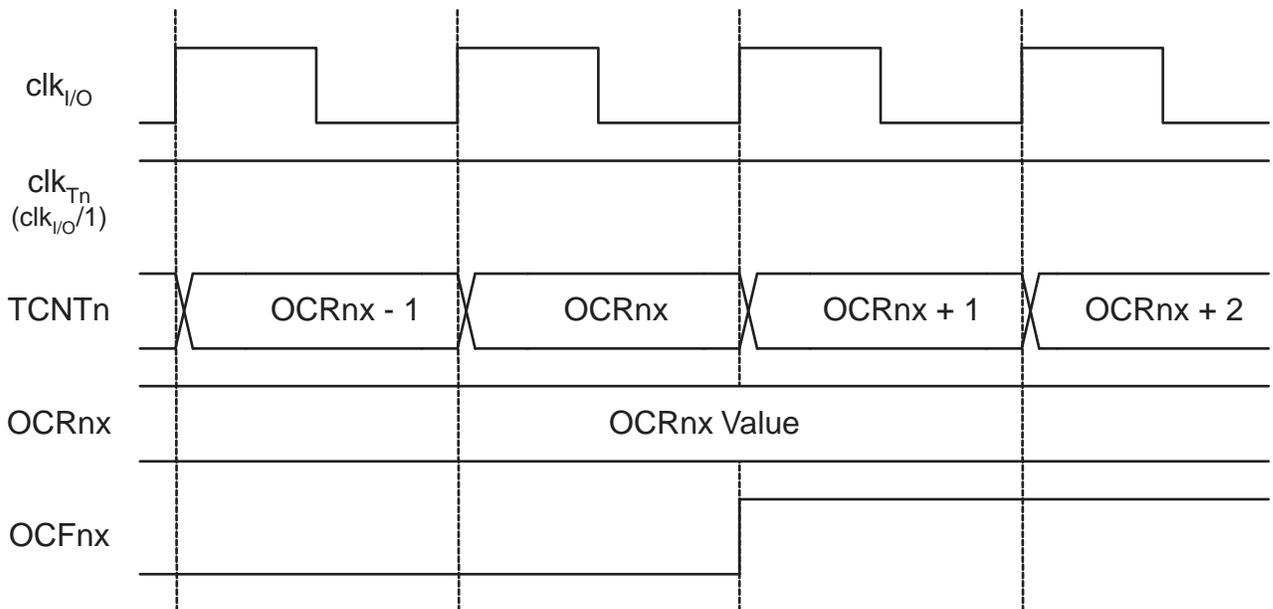
Figure 12-13 shows the same timing data, but with the prescaler enabled.
