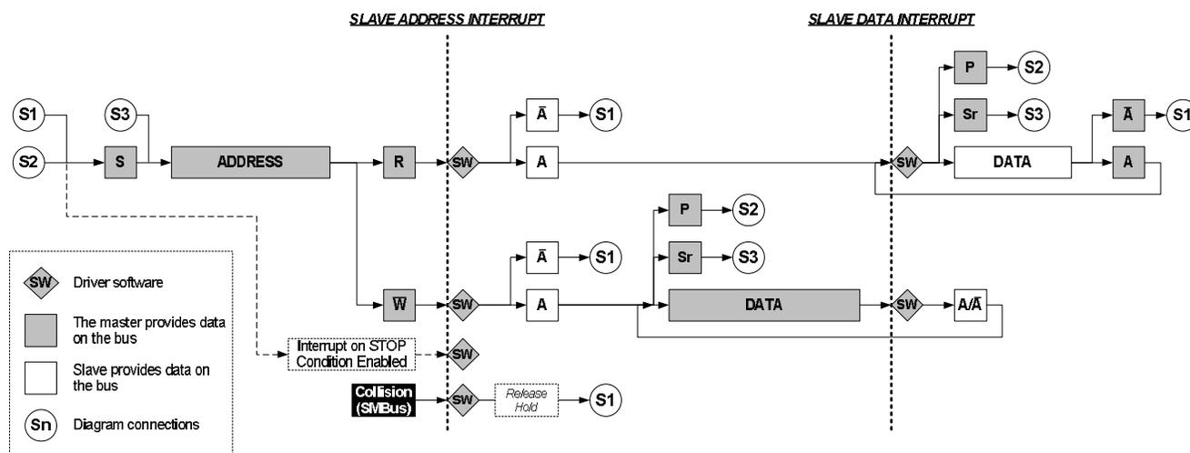
The number of interrupts generated is kept at a minimum by automatic handling of most conditions. Quick Command can be enabled to auto trigger operations and reduce software complexity.
