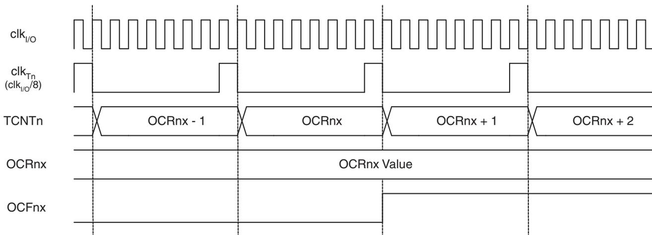
Figure 11-11 on page 69 shows the setting of OCF0A and the clearing of TCNT0 in CTC mode and fast PWM mode where OCR0A is TOP.
