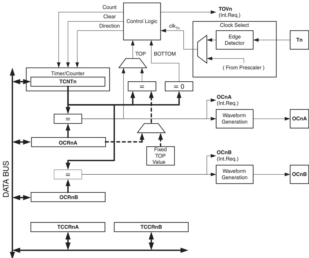
A simplified block diagram of the 8-bit Timer/Counter is shown in [Figure 11-1 on page 59](#). For the actual placement of I/O pins, refer to [Figure 1-1 on page 2](#). CPU accessible I/O Registers, including I/O bits and I/O pins, are shown in bold. The device-specific I/O Register and bit locations are listed in the “[Register Description](#)” on [page 69](#).
