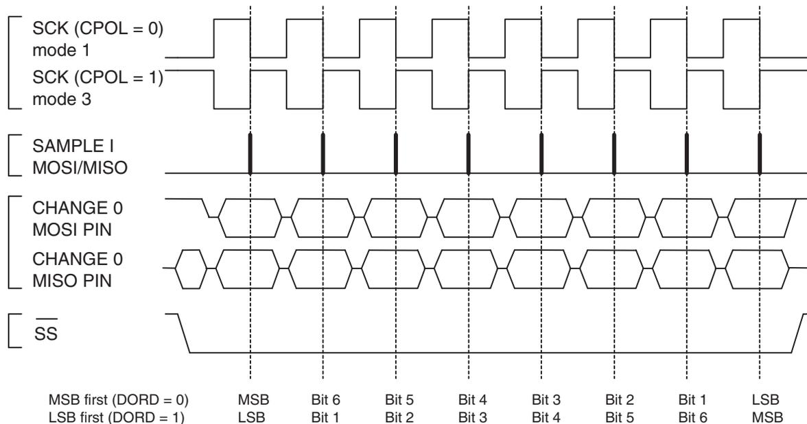
Data bits are shifted out and latched in on opposite edges of the SCK signal, ensuring sufficient time for data signals to stabilize. This is shown in [Table 16-2](#), which is a summary of [Table 16-3](#) and [Table 16-4](#).
