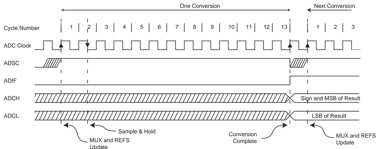
When Auto Triggering is used, the prescaler is reset when the trigger event occurs, as shown in [Figure 15-6](#) below. This assures a fixed delay from the trigger event to the start of conversion. In this mode, the sample-and-hold takes place two ADC clock cycles after the rising edge on the trigger source signal. Three additional CPU clock cycles are used for synchronization logic.
