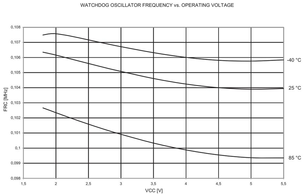
Figure 21-52. Watchdog Oscillator Frequency vs. Temperature
