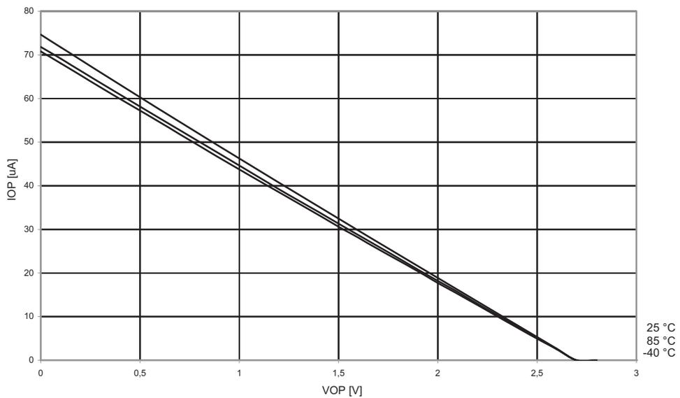
Figure 21-20. I/O pin Pull-up Resistor Current vs. Input Voltage ( $V_{CC} = 5V$ )
