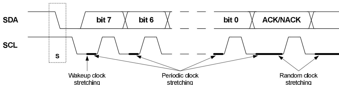
If the device is in a sleep mode and a START condition is detected the clock is stretched during the wake-up period for the device.
