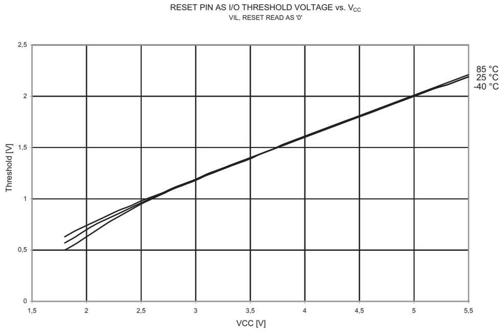
Figure 21-41.  $V_{IH}-V_{IL}$ : Input Hysteresis vs.  $V_{CC}$  (Reset Pin as I/O)
