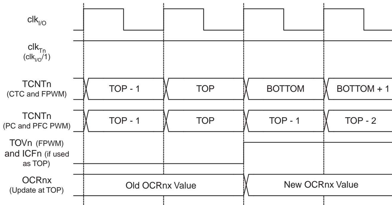
Figure 12-11 shows the same timing data, but with the prescaler enabled.
