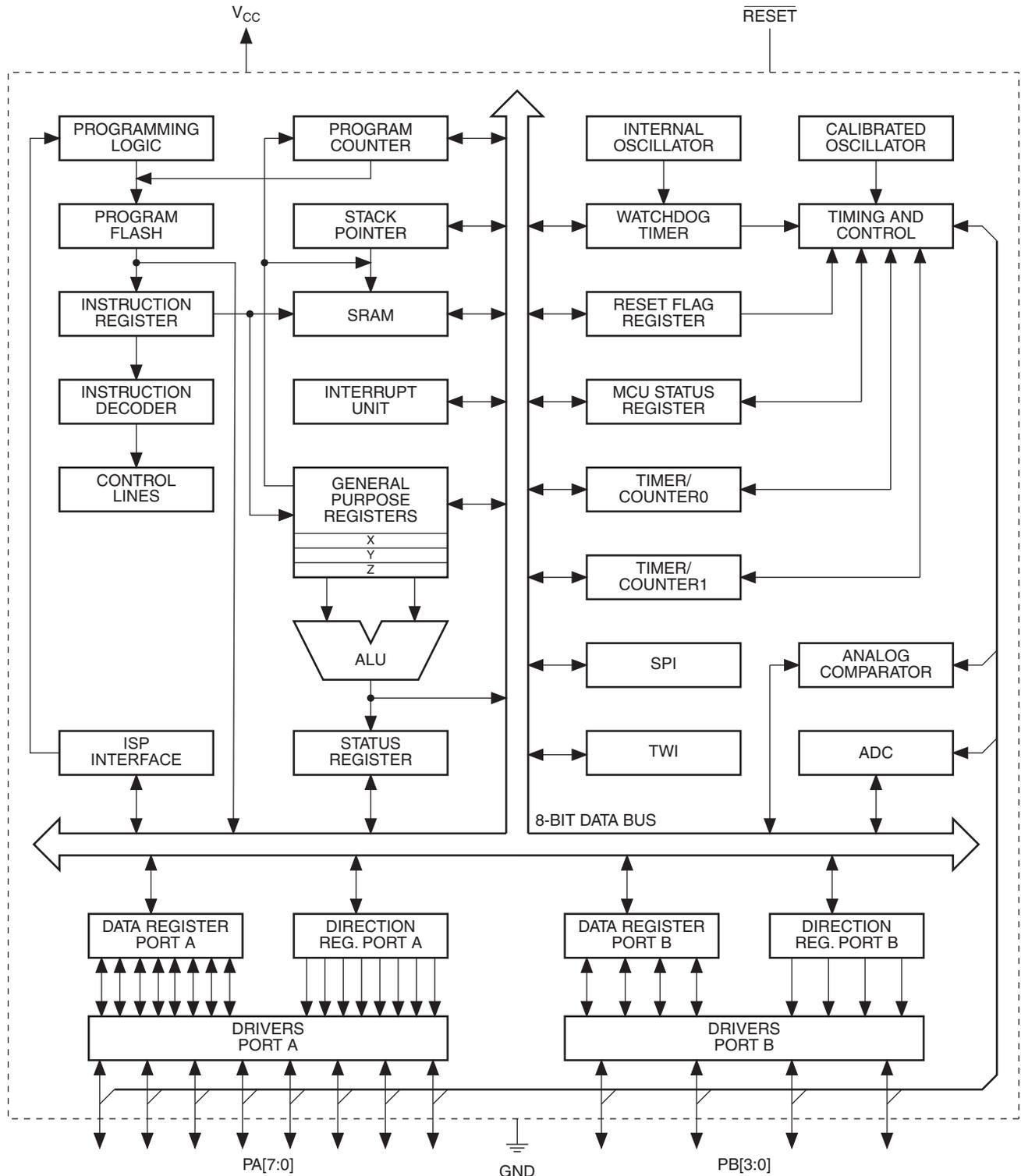
The AVR core combines a rich instruction set with 16 general purpose working registers and system registers. All registers are directly connected to the Arithmetic Logic Unit (ALU), allowing two independent registers to be accessed in one single instruction executed in one clock cycle. The resulting architecture is compact and code efficient while achieving throughputs up to ten times faster than conventional CISC microcontrollers.
