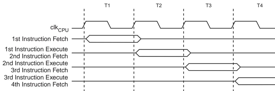
[Figure 4-4](#) shows the parallel instruction fetches and instruction executions enabled by the Harvard architecture and the fast access Register File concept. This is the basic pipelining concept to obtain up to 1 MIPS per MHz with the corresponding unique results for functions per cost, functions per clocks, and functions per power-unit.
