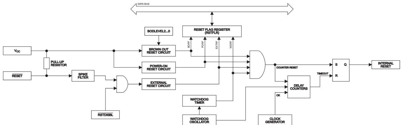
The I/O ports of the AVR are immediately reset to their initial state when a reset source goes active. This does not require any clock source to be running.
