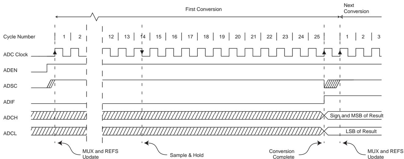
The actual sample-and-hold takes place 1.5 ADC clock cycles after the start of a normal conversion and 13.5 ADC clock cycles after the start of a first conversion. See [Figure 15-5](#). When a conversion is complete, the result is written to the ADC Data Registers, and ADIF is set. In Single Conversion mode, ADSC is cleared simultaneously. The software may then set ADSC again, and a new conversion will be initiated on the first rising ADC clock edge.
