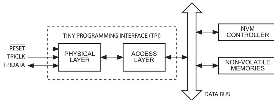
Programming is done via the physical interface. This is a 3-pin interface, which uses the  $\overline{\text{RESET}}$  pin as enable, the TPICLK pin as the clock input, and the TPIDATA pin as data input and output.
