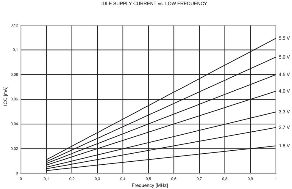
Figure 21-7. Idle Supply Current vs. Frequency (1 - 12 MHz)
