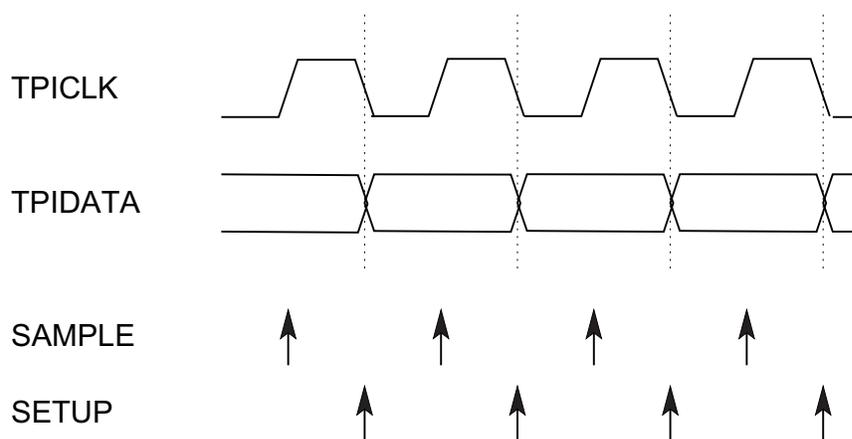
The TPI physical layer supports two modes of operation: Transmit and Receive. By default, the layer is in Receive mode, waiting for a start bit. The mode of operation is controlled by the access layer.
