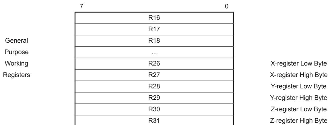
Note: A typical implementation of the AVR register file includes 32 general purpose registers but ATtiny20 implements only 16 registers. For reasons of compatibility the registers are numbered R16:R31 and not R0:R15.
