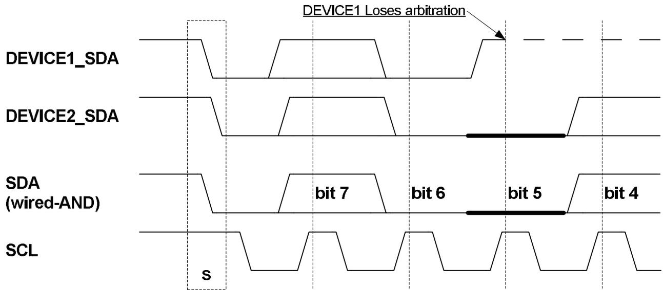
Figure 17-9 shows an example where two TWI masters are contending for bus ownership. Both devices are able to issue a START condition, but DEVICE1 loses arbitration when attempting to transmit a high level (bit 5) while DEVICE2 is transmitting a low level.
