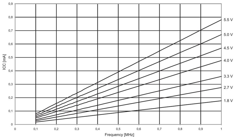
Figure 21-2. Active Supply Current vs. Frequency (1 - 12 MHz)
