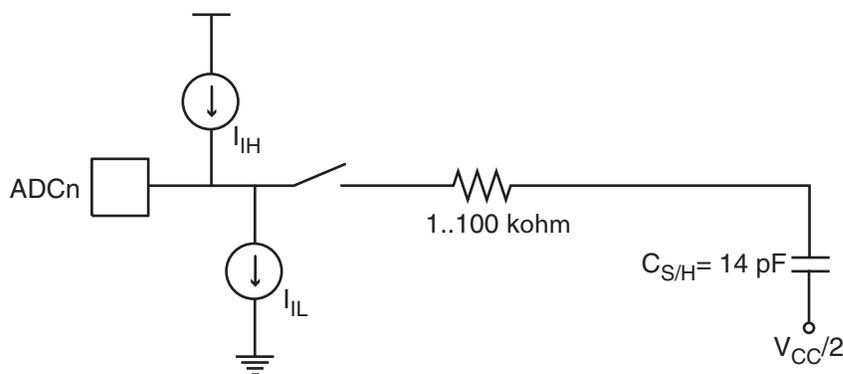
Note: The capacitor in the figure depicts the total capacitance, including the sample/hold capacitor and any stray or parasitic capacitance inside the device. The value given is worst case.
