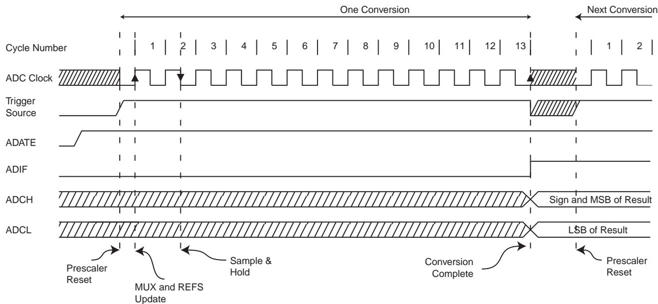
In Free Running mode, a new conversion will be started immediately after the conversion completes, while ADSC remains high. See [Figure 15-7](#).
