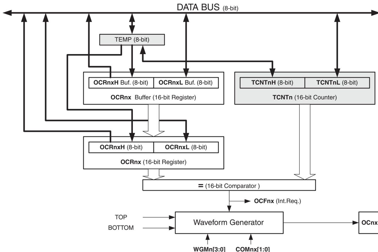
Figure 12-4 on page 81 shows a block diagram of the Output Compare unit. The small “n” in the register and bit names indicates the device number ( $n = 1$  for Timer/Counter 1), and the “x” indicates Output Compare unit (A/B). The elements of the block diagram that are not directly a part of the Output Compare unit are gray shaded.
