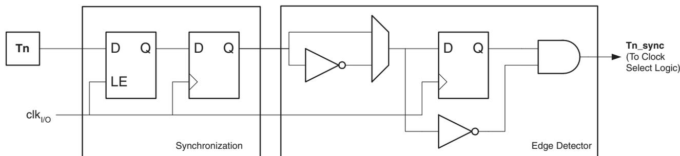
The synchronization and edge detector logic introduces a delay of 2.5 to 3.5 system clock cycles from an edge has been applied to the Tn pin to the counter is updated.
