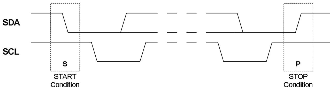
Multiple START conditions can be issued during a single transaction. A START condition not directly following a STOP condition, are named a Repeated START condition (Sr).
