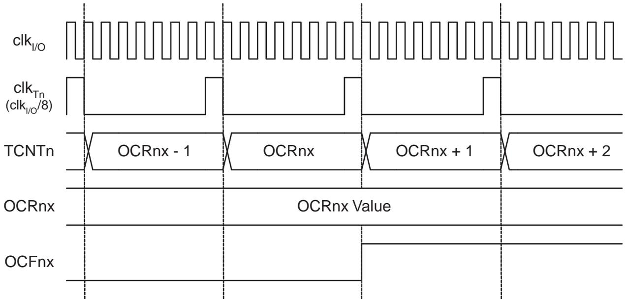
Figure 12-12 shows the count sequence close to TOP in various modes. When using phase and frequency correct PWM mode the OCR1x Register is updated at BOTTOM. The timing diagrams will be the same, but TOP should be replaced by BOTTOM, TOP-1 by BOTTOM+1 and so on. The same renaming applies for modes that set the TOV1 flag at BOTTOM.
