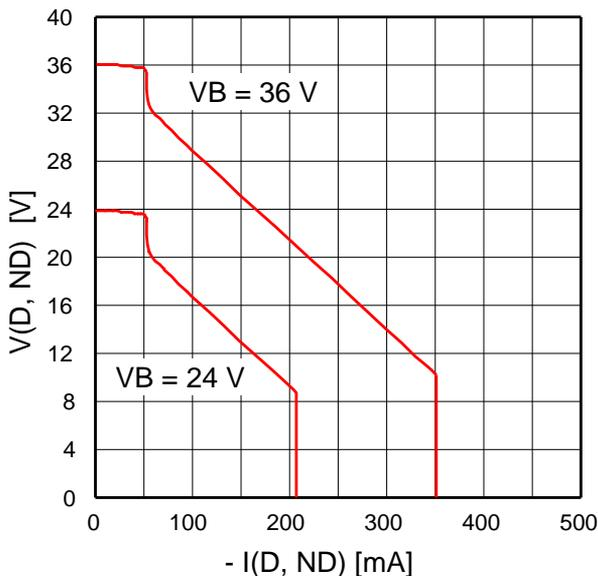
Figure 8: Load dependence of the output voltage
