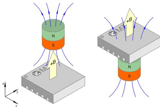
Figure 1: Example magnet positions in relation to iC-MZ
