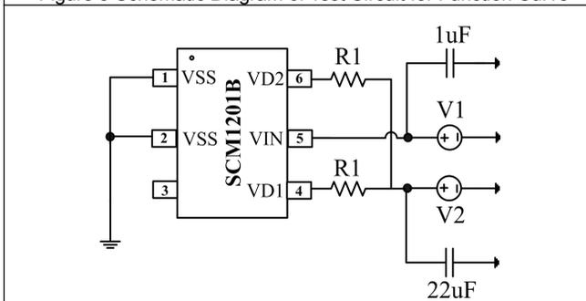
Figure 7 Schematic Diagram of Test Circuit for Switch Characteristics
