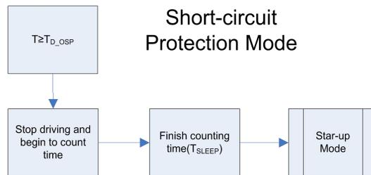
Figure 14 Flow Diagram of Short-circuit Protection Mode
