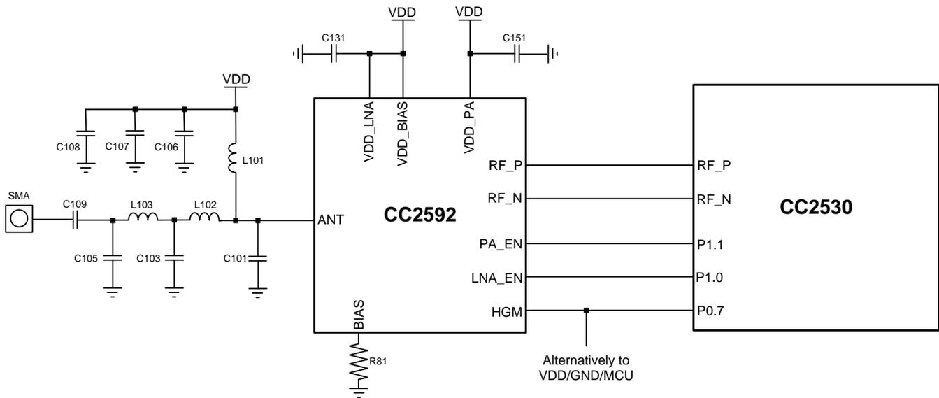
**Figure 9-1. Application Circuit Example for CC2530 + CC2592**
