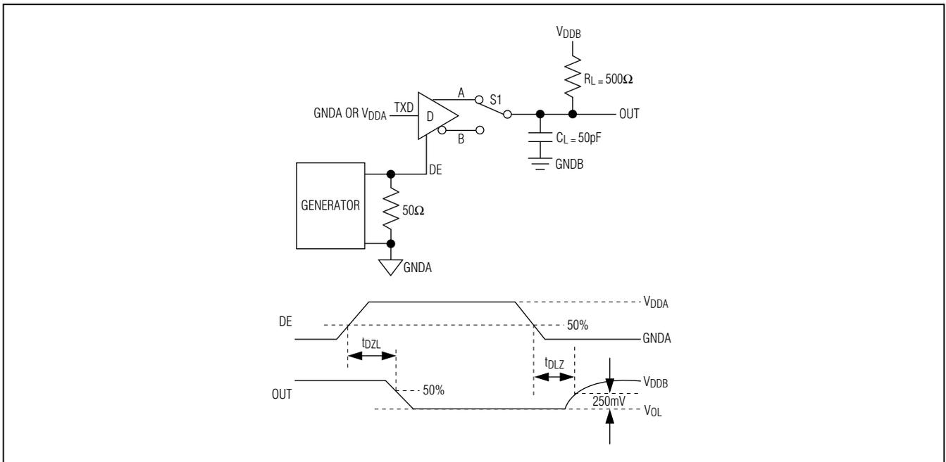
Figure 5. Driver Enable and Disable Times ( $t_{DZL}$ ,  $t_{DLZ}$ )
