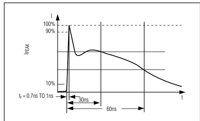
Figure 13. IEC 61000-4-2 ESD Generator Current Waveform
