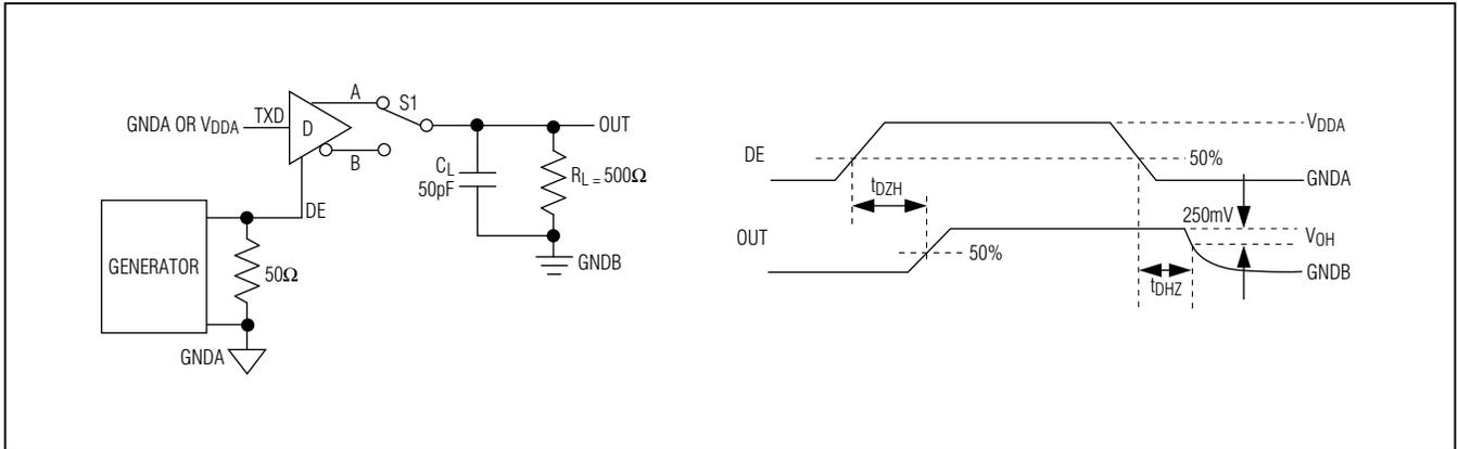
Figure 4. Driver Enable and Disable Times ( $t_{DZH}$ ,  $t_{DHZ}$ )
