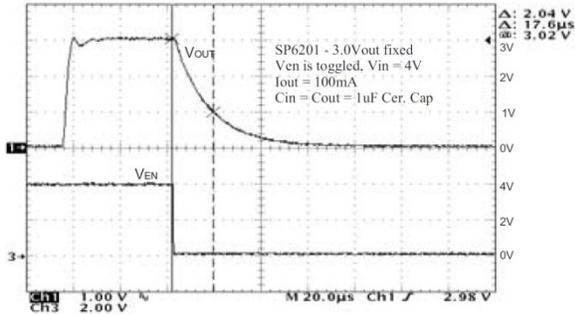
Fig. 28: Turn off time,  $I_o=100\text{mA}$ ,  $4V_{IN}$
