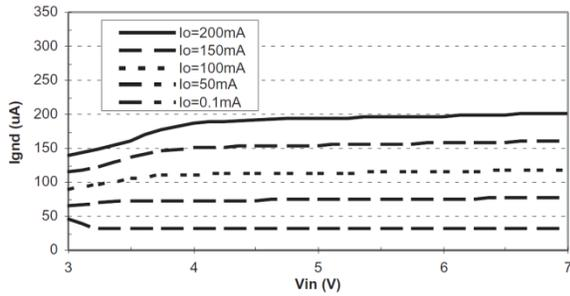
Fig. 10:  $I_{GND}$  vs.  $V_{IN}$  (SP6201 fixed 3.0V)
