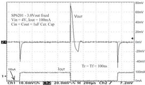
Fig. 32: Load Transient Response, 100mA step,  $4V_{IN}$
