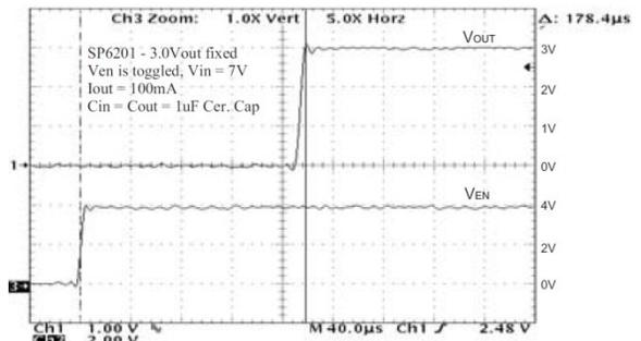
Fig. 25: Turn on time,  $I_o=100mA$ ,  $7V_{IN}$
