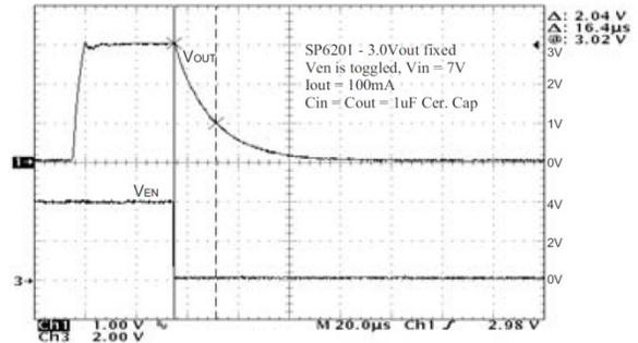
Fig. 29: Turn off time,  $I_o=100\text{mA}$ ,  $7V_{IN}$
