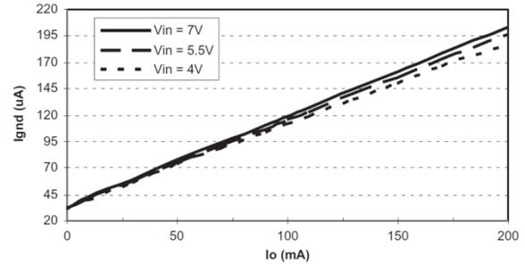
Fig. 11:  $I_{GND}$  vs.  $I_O$  (SP6201 fixed 3.0V)
