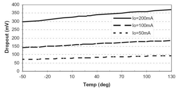
Fig. 5: Dropout vs. Temp (SP6201 fixed 3.0V)
