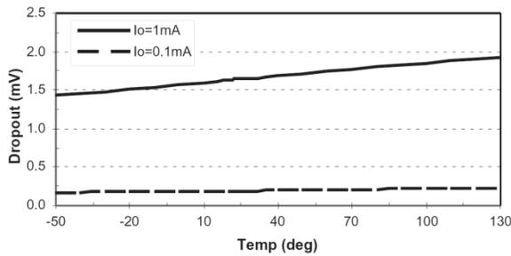
Fig. 6: Dropout vs. Temp (SP6201 fixed 3.0V)
