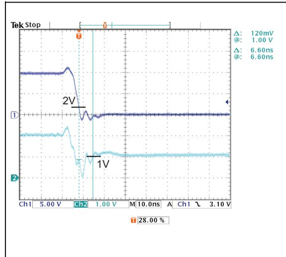
**FIGURE 3-7:**  $T_{ON}$  at  $V_A = 10V$ .
