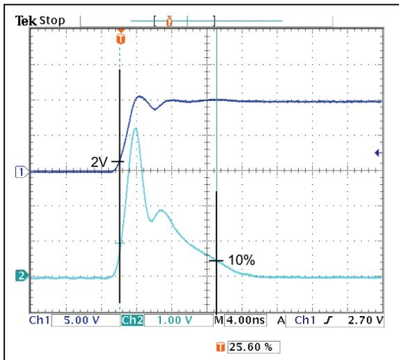
**FIGURE 3-4:**  $T_{OFF}$  at  $V_A = 10V$ .
