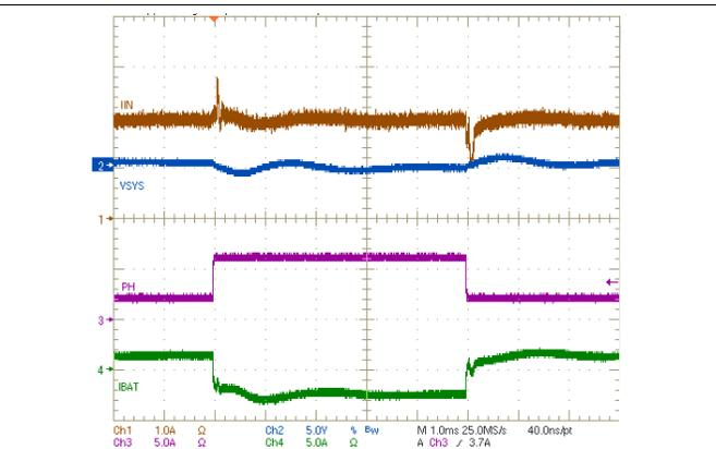
CH1: input current, 1A/div; CH2: system voltage (AC), 5V/div; CH3: system load, 5A/div; CH4: battery charge current, 5A/div, 1ms/div
