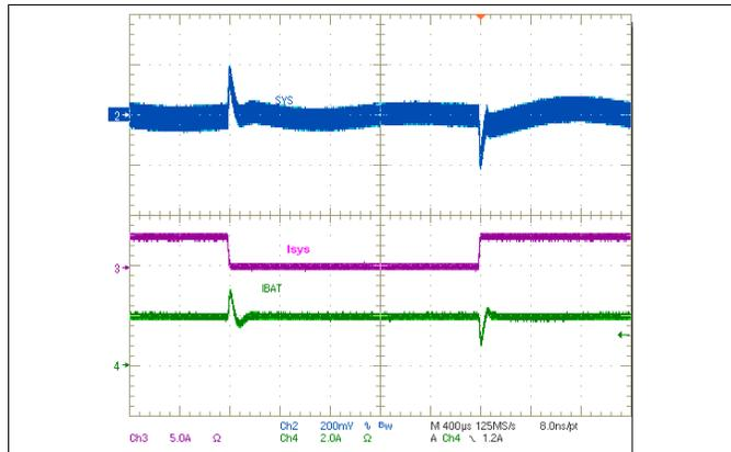
CH2: system voltage (AC), 200mV/div; CH3: system load current, 5A/div; CH4: battery charge current, 2A/div, 400us/div
