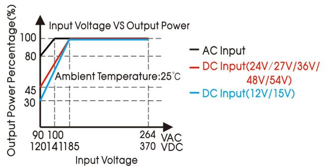
Note: With an AC input voltage between 90-100VAC and a DC input between 120-185VDC the output power must be derated as per the temperature derating curves.
