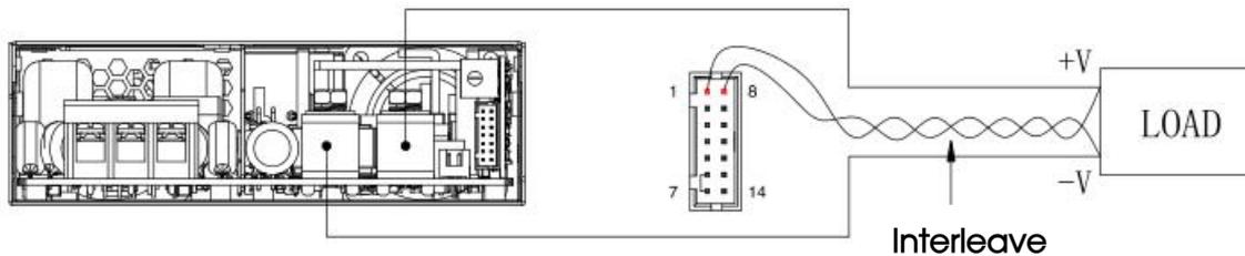
Note: 1. VS+ and VS- cannot be shorted or reversed, otherwise the power module will be damaged.
