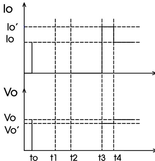
$t_0-t_1$  moment: The output current is nominal  $I_o$ , and the output voltage is nominal  $V_o$ ;
