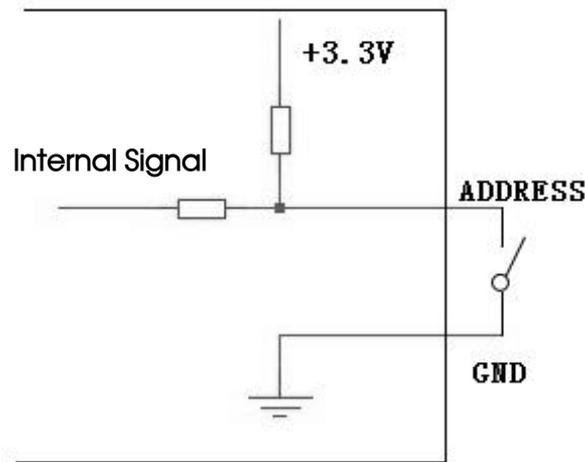
The internal pull-up resistance value of the power module is 10k $\Omega$ , and the external impedance can be matched according to the actual application to meet the high and low voltage range.
