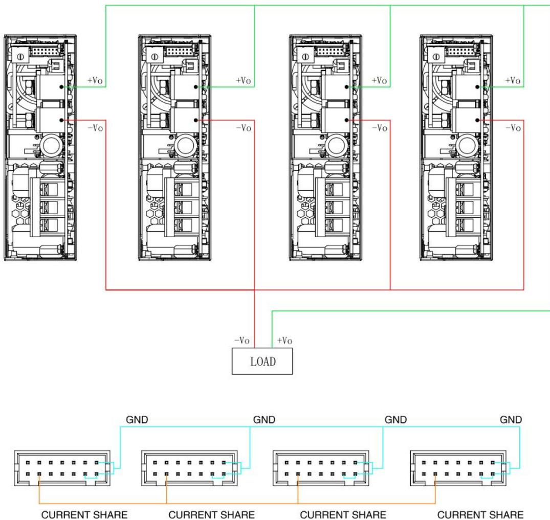
Note: 1. When using in parallel, the number of parallel modules cannot exceed 4.
