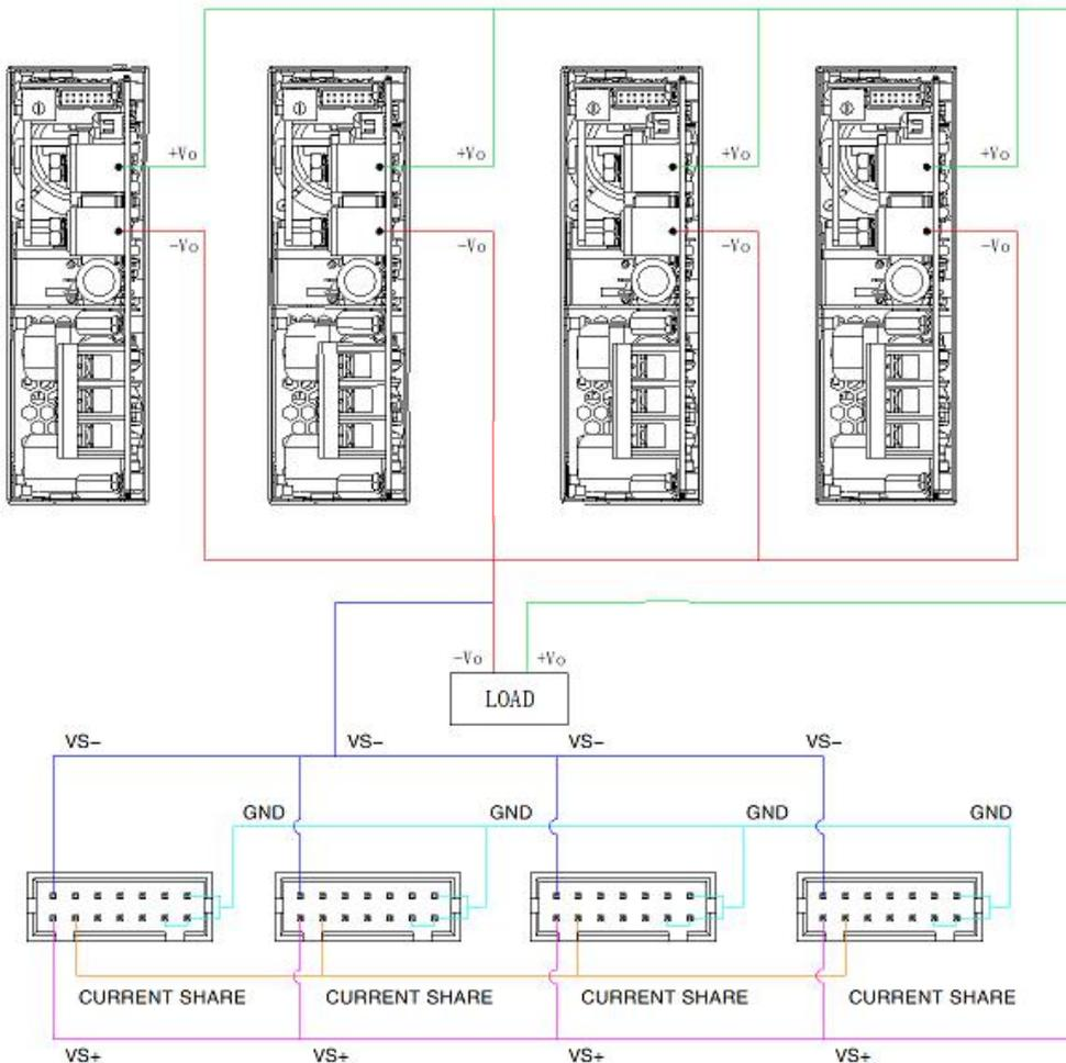
Method 2: Only the current sharing bus is connected, and the remote compensation is not connected.
